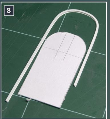
8. After the styrene beam cools, it will stay in its designated shape, and can be easily attached to the turntable bridge without any tension.
