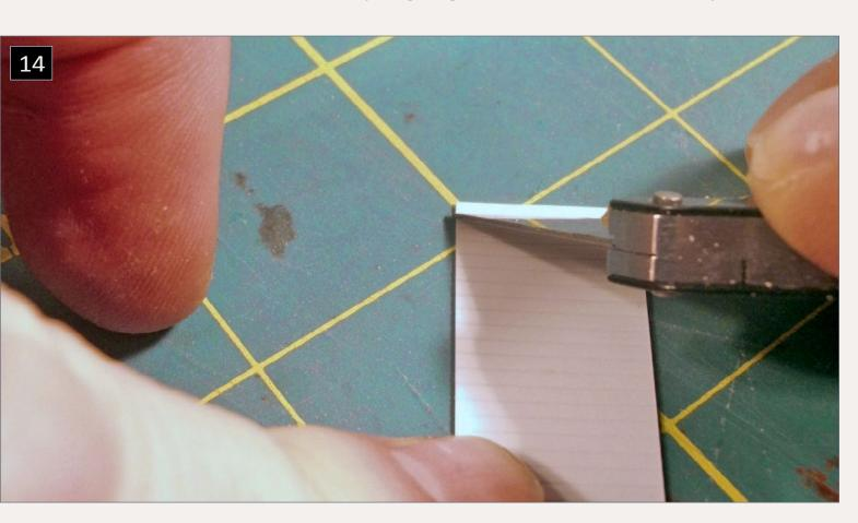
14. Photo showing how to cut the strip styrene for the horizontal bracing on the feed bin.
