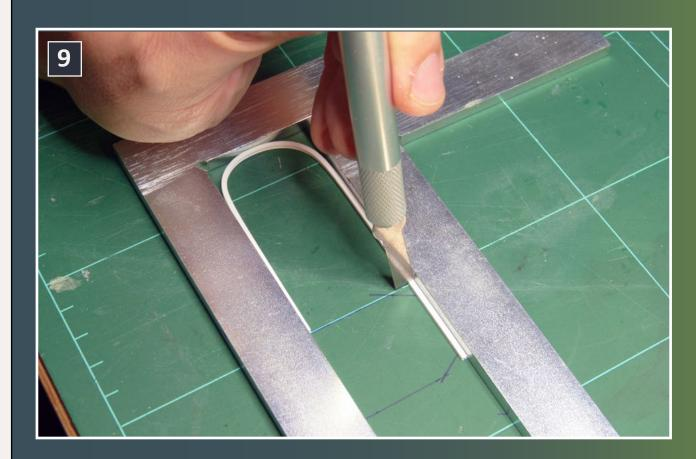
9. I cut the arch to length with a sharp blade.
