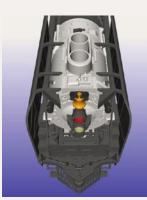
The 14-wheel N scale Centipede tender will have a unique articulated mechanism to permit operation on 11" radius curves.
