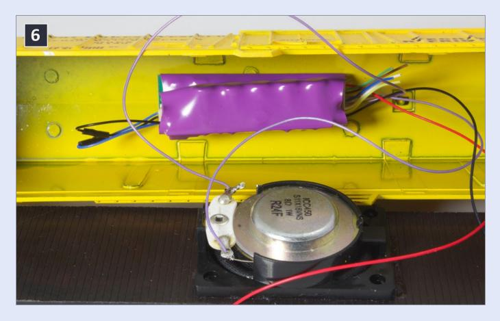
6. Interior view of SoundCar and CurrentKeeper installed in a 50-foot HO box car. Bruce Petrarca photo.
