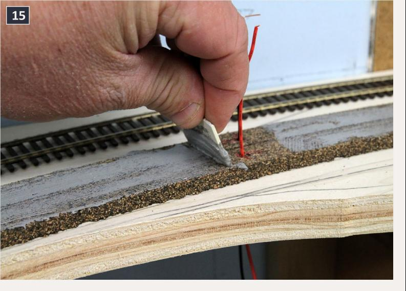
15. Flooring installers lay linoleum or tiles using notched trowels to apply just the right amount of mastic to the floor. If it's good enough for them, it's good enough for me. My home-made trowel leaves little ridges of caulk behind, enough to hold the track, but not so much that the track floats in the stuff.
