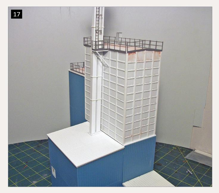
17. View of the completed main structure with feed bin attached and elevator installed.
