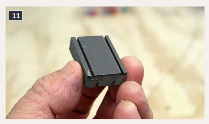
11. This simple tool from MLR Mfg. costs only a few bucks and makes shaping ME flex track into curves easy.
