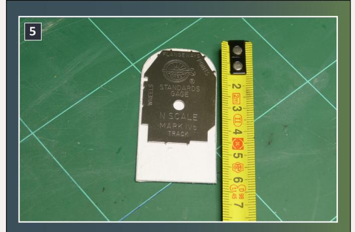
5. The arch template in comparison with a standard N scale track gauge. The top radius fits inside the profile – so motive power will fit beneath the arch.
