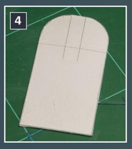
4. The final arch template. I used scissors to cut the styrene exactly along the printed line.
