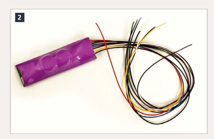
2. SoundTraxx Tsunami SoundCar DCC decoder. SoundTraxx photo.
