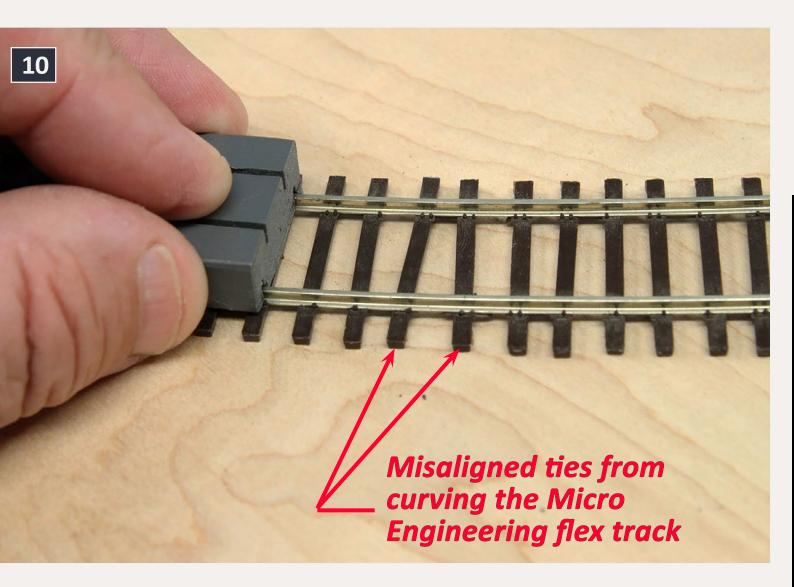
10. Curving ME track often results in the ties losing position and becoming misaligned. I work the ties back into alignment once the track is laid.
