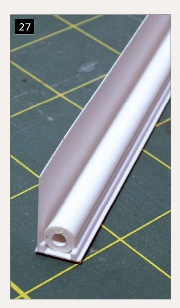
27. Step 2 of the auger construction showing the partially assembled auger with the .010" styrene ready to wrap around the tubing to form the U-shaped auger.
