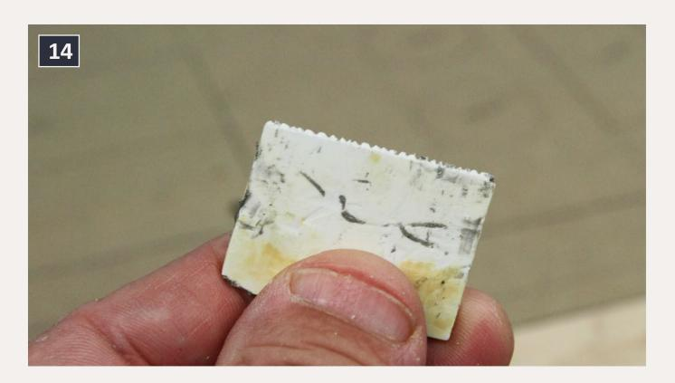
14. I use this homemade itsy-bitsy notched trowel to spread caulk. After almost 15 years of use, it may be getting to be time to make another one. It started as a small scrap of .060" styrene. I sharpened one edge like a chisel, then made notches with a tiny triangular jeweler's file.
