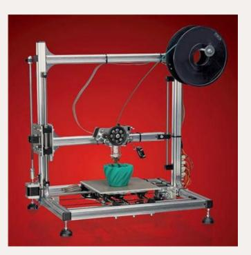
Micro-Mark (micromark.com) is selling a Velleman model K8200 3D printer at \$724.95. It is intended for use by intermediate to experienced craftsmen. The printer creates objects up to 7.87 x 7.87 x 7.87 inches by laying down (printing) multiple micro-thin layers of melted plastic less than .010 inch thick. The system uses FFF (fused filament
