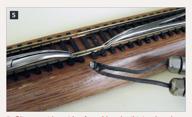
5. Clips on either side of a soldered rail joint draw heat away from the work and keep plastic ties from melting. Ronald D. Smith photo.
