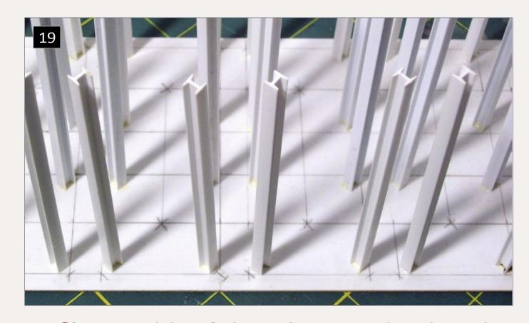
19. Close-up of the silo base showing grid markings for silo centers. The silos are space 1.5" on-center.
