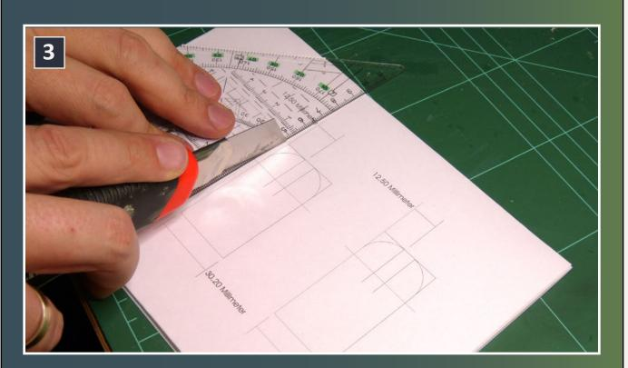
3. I used a sharp knife and a ruler to cut out the arch template. Then I removed the backing paper and affixed the paper to a piece of styrene.
