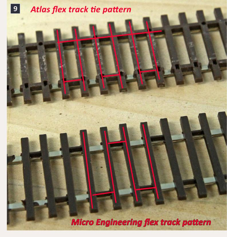
9. Note the different tie patterns of Atlas and ME flex track. Atlas track is designed to curves smoothly but won't hold its shape. ME track is trickier to curve smoothly but once curved holds its shape.
