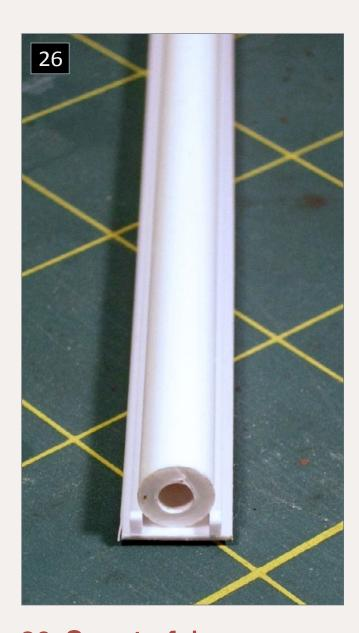
26. Step 1 of the auger construction showing the partially assembled auger. Note .030" by .040" styrene strips laid against either side of the ¼" tubing and flat top to support the .010" styrene wrapped around the tubing to form the U-shaped auger profile.
