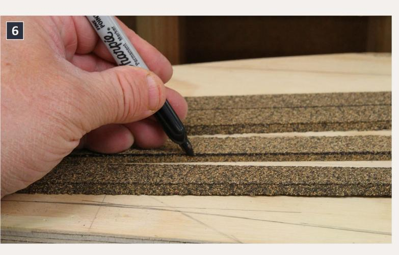
6. Marking the edge of the cork strips before installation makes the seam where they join obvious to the casual observer. I use a black Sharpie marker.
