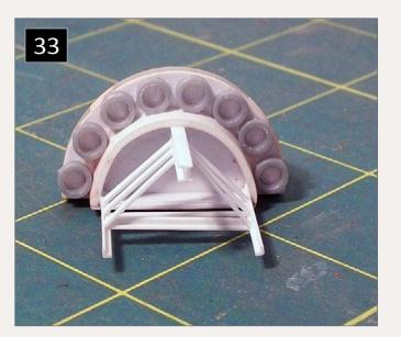
33. This bottom view of the elevator distributor head shows the legs constructed of two pieces of 0.060" angle and one 0.080" H-column. The legs rest against a piece of 0.040" thick by 0.188" high styrene piece wrapped around the base, and offset just enough to
