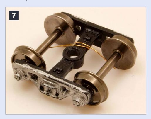
7. Detail of the power pickup on the trucks, ready to mount and solder feed wires to them. Hint: Make sure the insulated sides of the wheels are on the same side of the truck. Bruce Petrarca photo.
