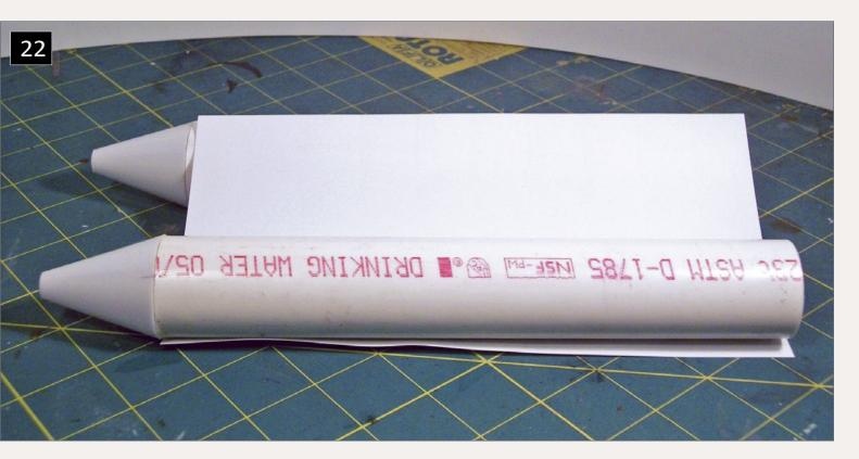
22. This photos shows the styrene temporarily tacked with CA cement to the PVC silo. The next step is slowly wrap the styrene around the PVC spreading CA cement every half inch and firmly pressing the styrene against the PVC to prevent bubbles from getting between the PVC and styrene.
