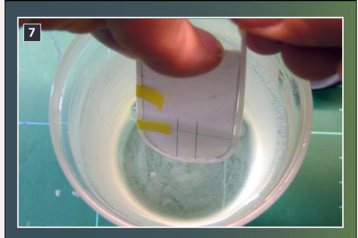
7. I dipped the beam into the boiling water for about a minute, then pulled the loose side around the template to bring the beam into shape until it cooled.
