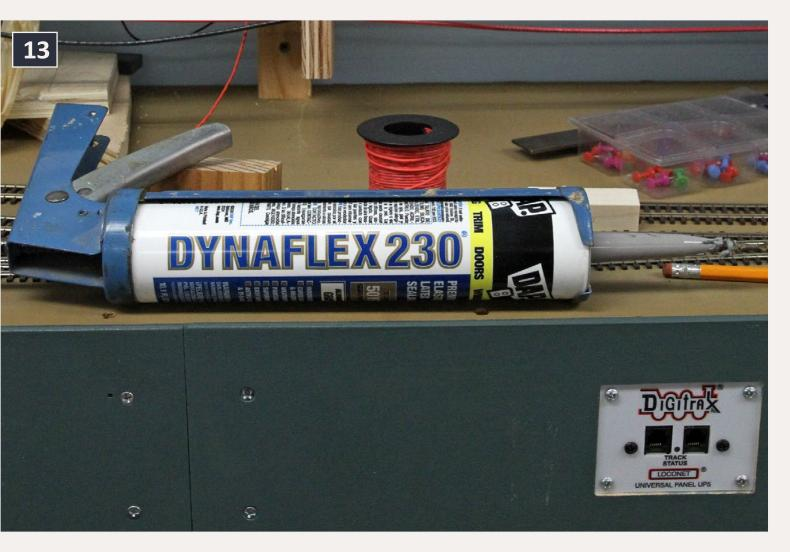
13. I use paintable latex caulk to glue down ME flex track. I prefer gray because it more or less matches the ballast color. I got this tube from a local big-box store. Once the track is bedded in this stuff I have about 10 or 15 minutes of working time.
