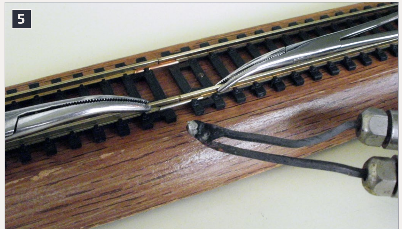
5. Clips on either side of a soldered rail joint draw heat away from the work and keep plastic ties from melting. Ronald D. Smith photo.
