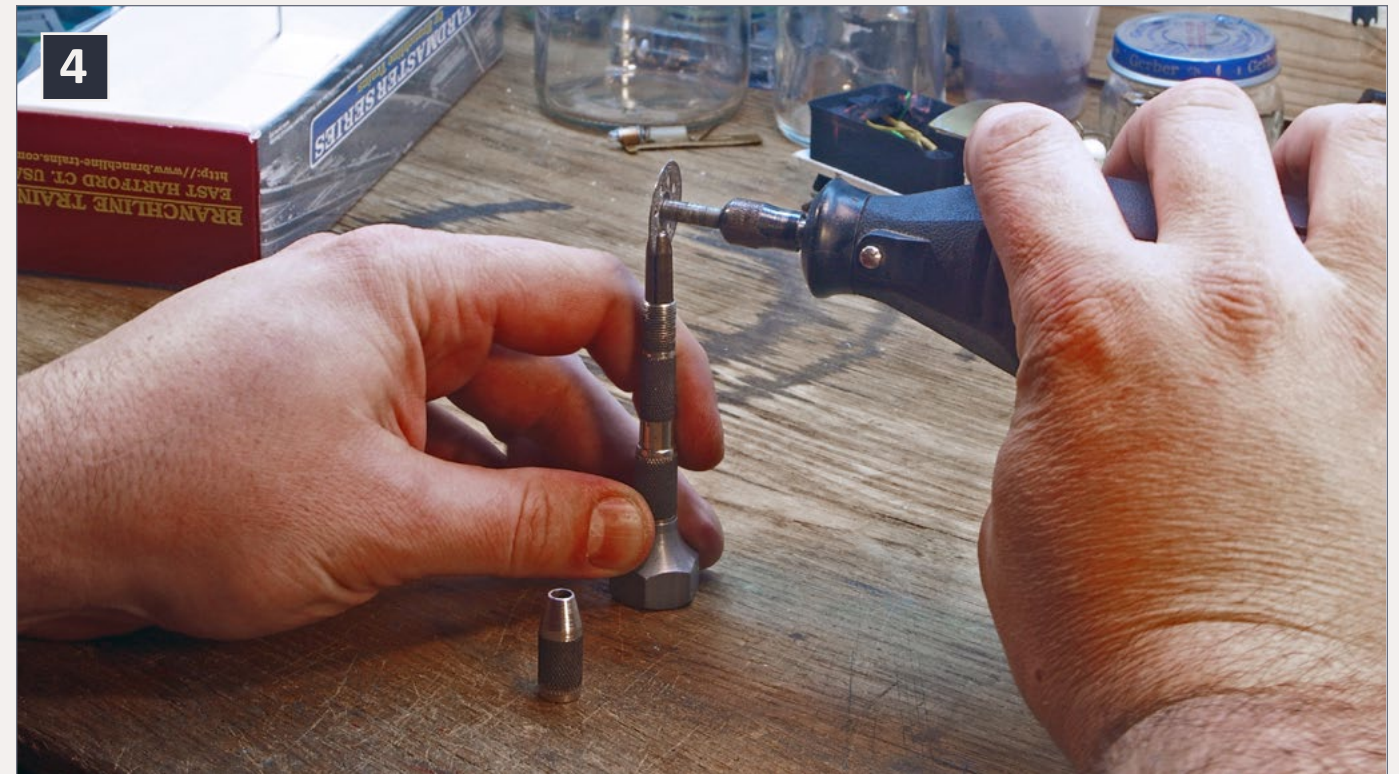
4. A thin diamond blade refaces worn pin vise collets. Ken Rickman photo.
