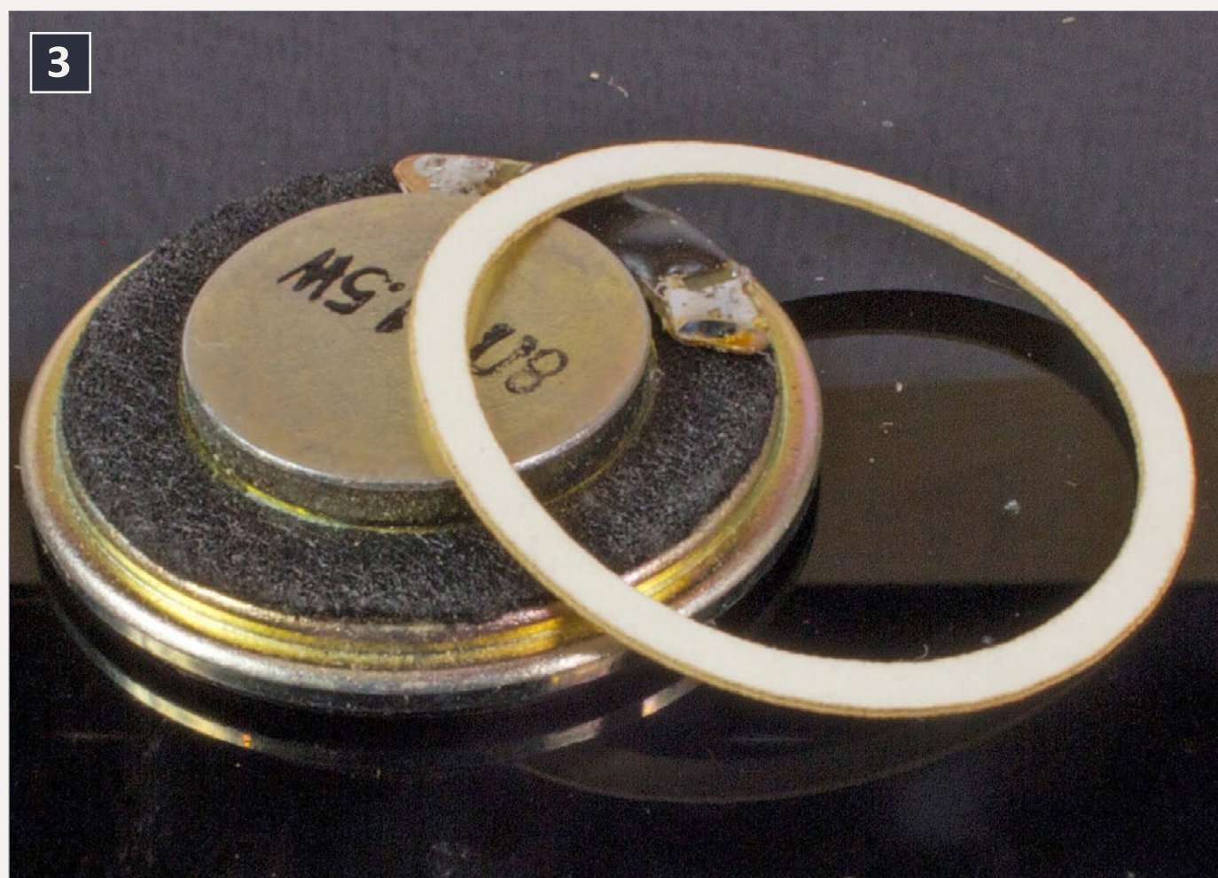
3. Gasket shown with a 28 mm round speaker.
