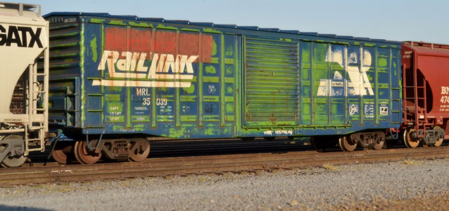
8. Jeff Meyer ends this month's video with one of his recent Montana Rail Link creations. This Rail Link car's paint is simply washing off the Burlington Northern green freight car. Lots of careful wet sanding produced the effect.
