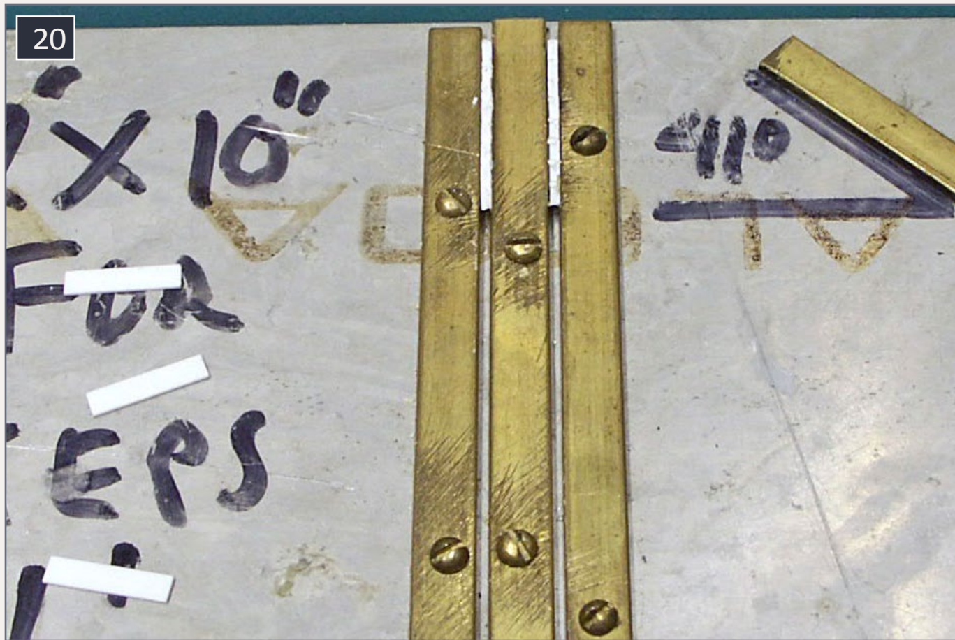
20. Part of the stair jig is this section I made to hold the stringers while the treads are cemented to them. This fixture is a must, as it is almost impossible to cement the treads to the stringers without it.
