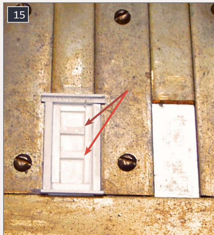
15. The rest of the door rails have been added creating the three panels needed for the door.
