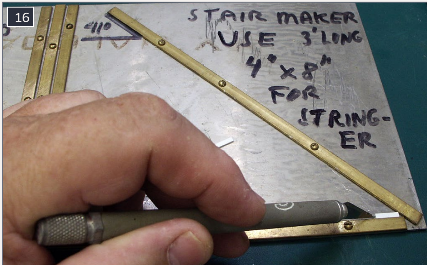
16. I made this jig for building stairs. The jig is at 41° typical of many stairs. I also made notes on the base so I wouldn't have to remember the sizes needed every time I made steps.
