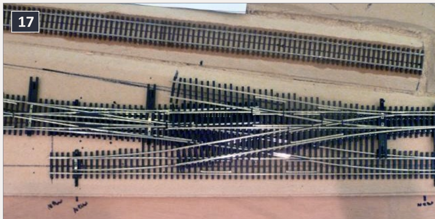
17. The switches temporarily laid in place.
