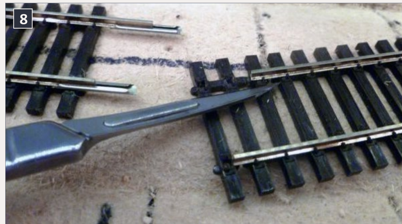
8. Trimming spikes for the rail joiner.
