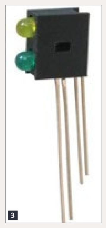
3: A bi-level LED assembly suitable for a track-side signal as is. Photo courtesy of All Electronics. signal will show the straight route when the turnout is still set for the diverging route.
