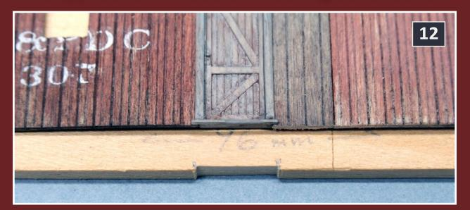
12: The door casting is thicker than the sheathing. To accommodate the door casting, notch the edge of the floor.
