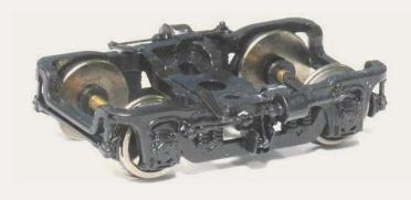
A popular four-wheel passenger truck with insideswing hangers was General Steel Casting's model 41-N-11 (above). Rapido's HO scale version, item 102012,
