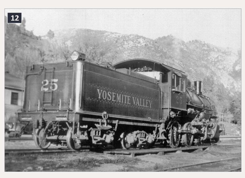
12: This photo of the 25 in El Portal shows the marker brackets on the rear of the tender along with flag holders for extras and sections when running in reverse. Two brakeman lanterns and a pair of markers are stored on the back wall of the cab above the canvas curtain. – *Fred Stoes photo.*
