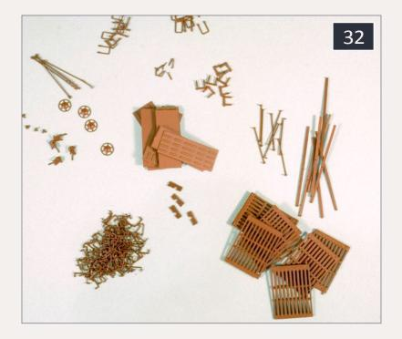
32: It's a long way from the pile of parts to the finished car body in 33. The grabirons took roughly 40 minute per car to glue in place.
