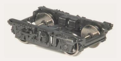
One of the most common outside-swing hanger fourwheel passenger trucks for both new and rebuilt cars after 1947 is the 41-BNO-11 (above). The prototype was built by both General Steel
