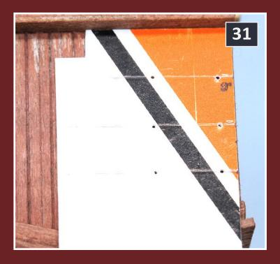
31: Use a piece of scrap card stock to make a drilling template for the end ladders. The template is set up for Westerfield 23" straight grab irons spaced 18" apart. Position the template and mark the drill locations.
