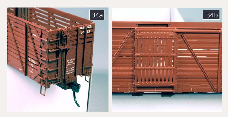
34a-34b: Left: The brake platform assembly turned out to be the most troublesome part of the kit, as the parts didn't fit as well as the rest of the kit. The end of the car with all of the grabirons in place. Right: The door detail.
