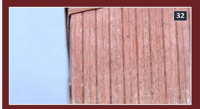
32: Lightly twist a #78 drill and lightly drill at each hole in the template, drill just enough to mark the surface of the sheathing. After removing the template, find your marks and drill the holes to depth.
