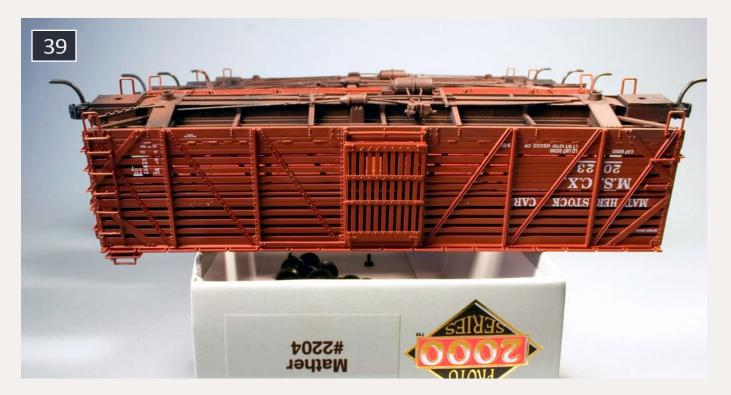
39: A completed stock car body except for trucks and a final road test. The last step after installing trucks and road testing, will be to add some more weathering.
