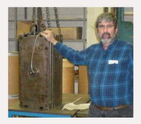
Bowser's production manager stands next to massive injection mold for HO scale Alco locomotives scheduled for release later this year. The steel mold will be installed in a new 110-ton fully computerized all-electric injection molding machine recently acquired by Bowser.
