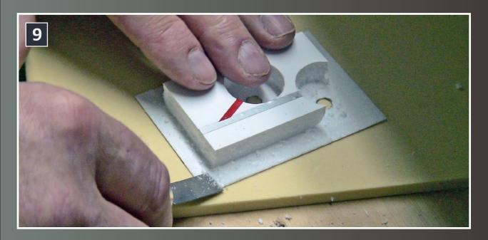
Using a 1/2"-wide flat X-Acto blade, carefully scrape the filler off the veneer to allow the panel to set flat on the fascia.
