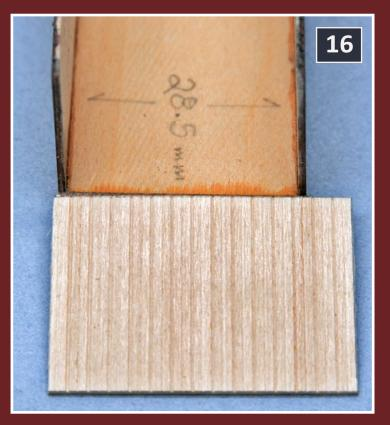
16: The ends are fabricated from siding material. Use the completed car body to determine the exact width required for each end. Do not assume that they are both the same width. In theory they should be, but it is likely they will differ slightly.
