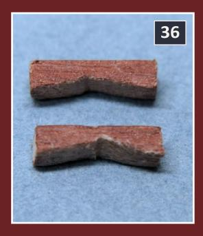
36: Cut two pieces of scale 6x6 stripwood 24" long. Notch the underside to match the slope of the roof.
