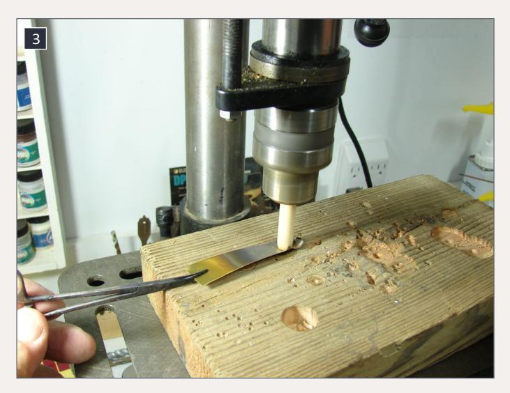
3. The reflector is formed by forcing a slowly-turning dowel into the annealed brass plate.
