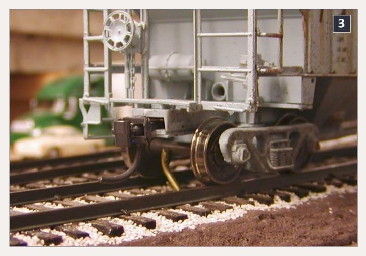
3: Joe Atkinson's brakes disengage automatically – the wire falls back in the hole when the car is pulled away. Joe Atkinson photo.
