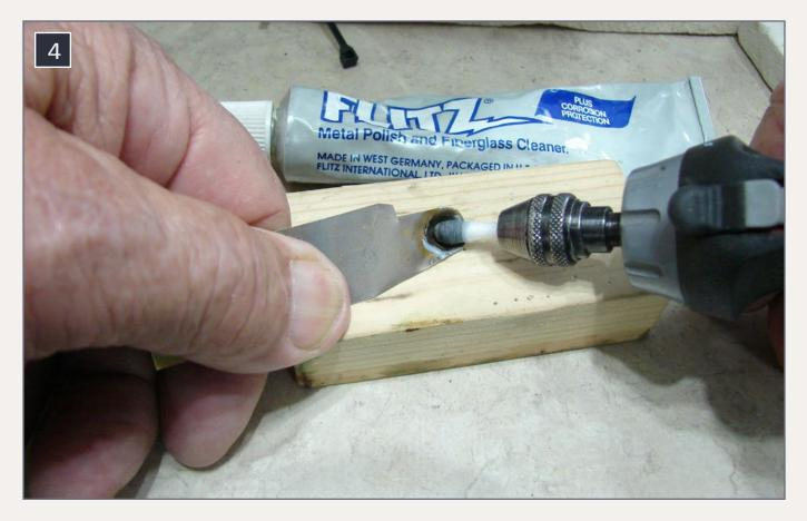
4. A rotary tool, Q-tip, and Flitz polish are used to create a shiny reflector.
