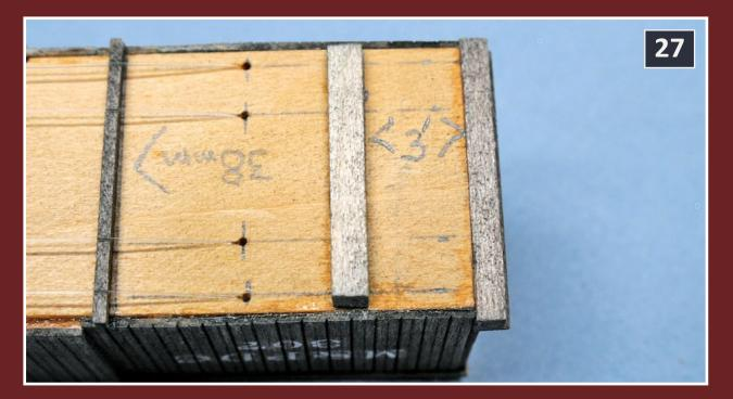
27: Create two bolsters from scale 6x12 stripwood. Glue in place 3' from the car end. Paint the underbody and truss rods black.
