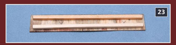
23: Glue another support strip along the peak edge of the roof segment. Offset this one about 1/8" from the edge. It will need to clear the one added to the peak of the opposite roof section.
