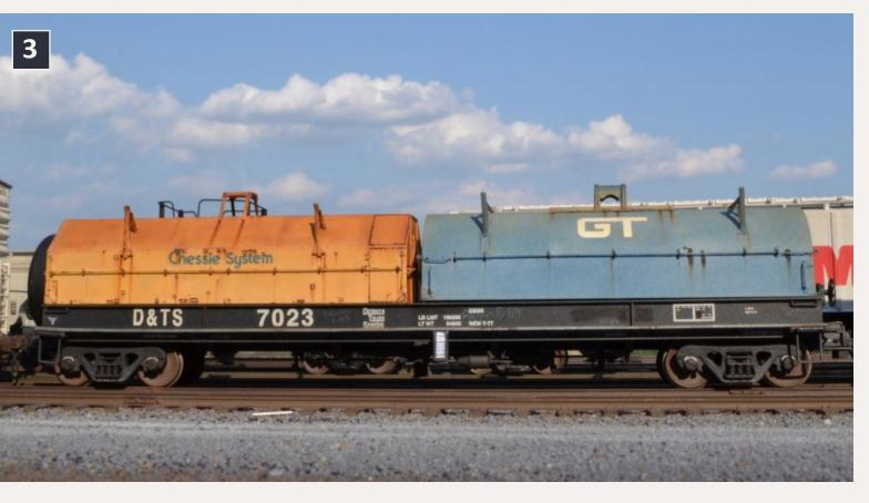
3: A Red Caboose coil car is re-detailed with new brake rigging, grab irons, pin lifters, air hoses and Sergent couplers. The hoods are heavily faded using an airbrush and white oil paints. The rest of the weathering is done by hand with oil paints and powders, to closely match prototype photos.
