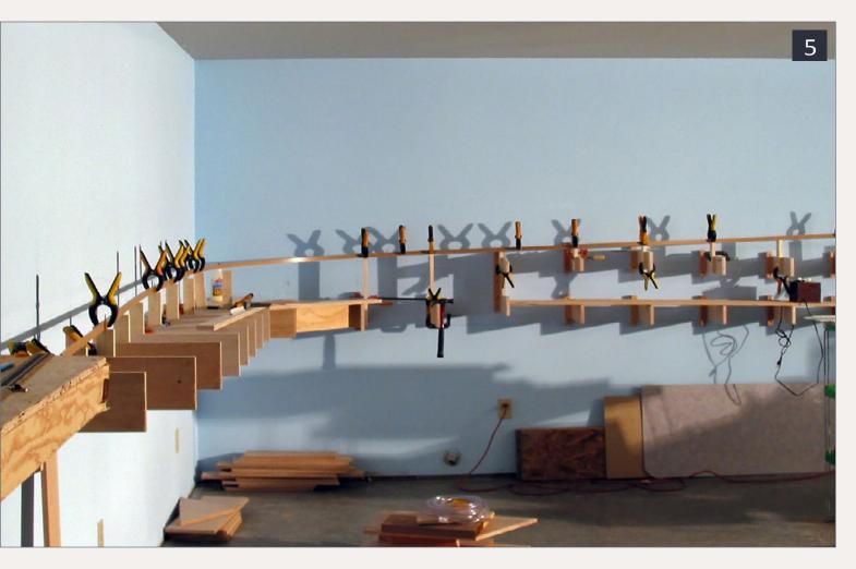
5: In the beginning was Mill Bend (the recycled Mill City from the previous layout), nearest on the extreme left. In mid-January 2004, Masonite spline roadbed installation was going gangbusters heading for Oakhill (top) and Redland (bottom). Clamping all those splines needs strong wrists!
