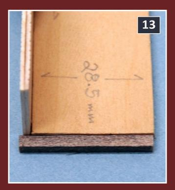
13: Fabricate the end sills from a scale 10x10. Cut it three scale inches longer than the width of the car (floor, two sides plus 3").
