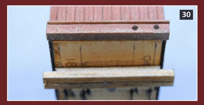
30: Drill #72 holes in the middle of the end sill, aligned with the truss rods. Add Grandt 5093 NBW castings. Paint them black.
