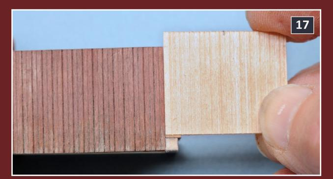
17: Using the side sheathing for the ends creates a roof peak one foot above the eave. Mark the eave height on both edges of the end. Determine the center of the end, and cut the roof slopes.
