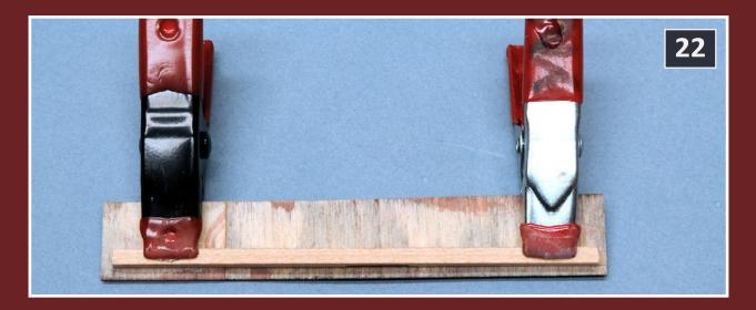
22: Measure the exact width of the roof from the peak to the eave; on my model it is 16mm. Cut the roof segments to this width. Glue two segments end-to-end. When dry, cut this piece to match the length of the body, allowing for a very slight overhang on the ends. Glue a roof support (1/8" square stripwood) along the eave edge of the roof sheet. Set it back from the edge 1.6mm.
