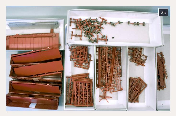
26-27: All of the parts for our stock car build are sorted into boxes. Kit boxes work well for this. The photo on the right shows the sort for a build of 12 refrigerator cars – notice that the car ends with the reporting marks and car numbers are kept with the corresponding car body.
