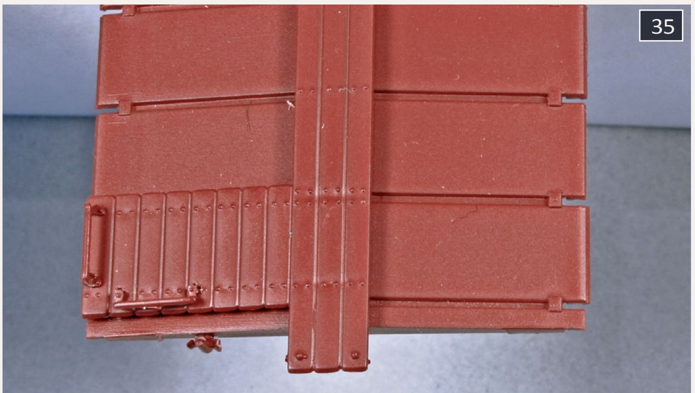
35: The grabiron detail and the retainer valve on the roof assembly.
