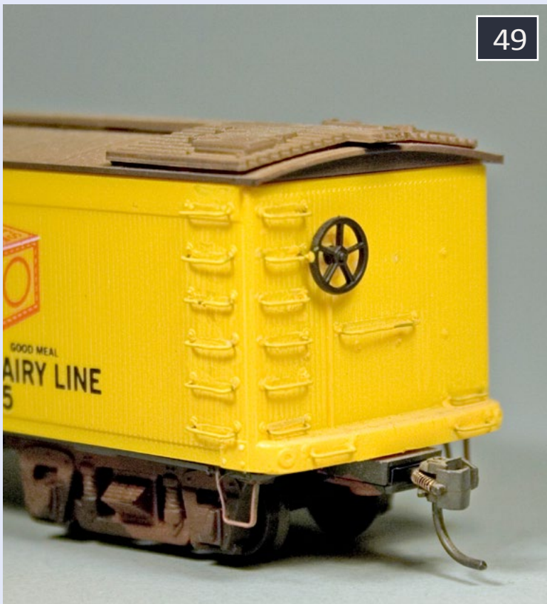
49: An MDC milk reefer detail upgrade. Notice the wire grabs and the more delicate stirrups on the upgraded version.
