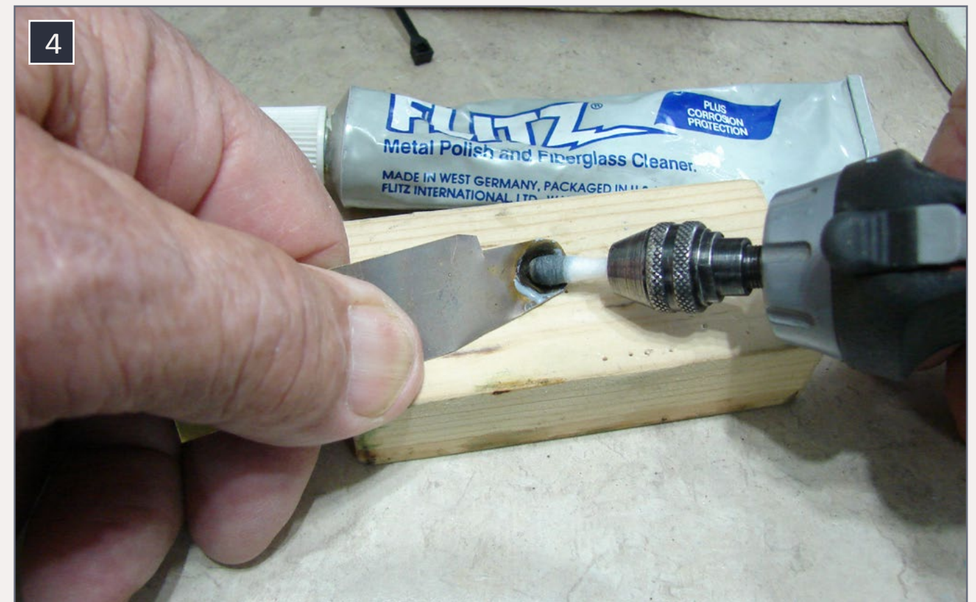
4. A rotary tool, Q-tip, and Flitz polish are used to create a shiny reflector.
