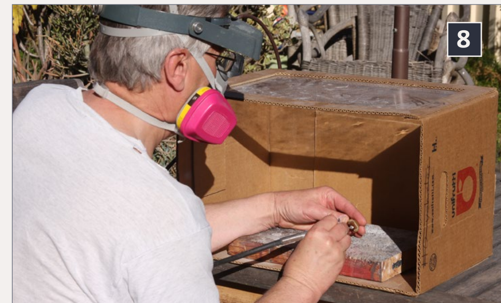
8: Charles Hepperle's converted apple box contains dust and overspray from modeling projects. A clear-plastic sunroof lets in some light.
