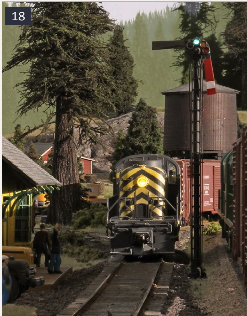
18: The lower quadrant train order semaphore at Oakhill. The Oakhill operator has set the eastward semaphore blade to stop (up/horizontal) while copying an order for an eastward train. This ensures the train won't pass the station before the order can be prepared. Tam Valley Dual
