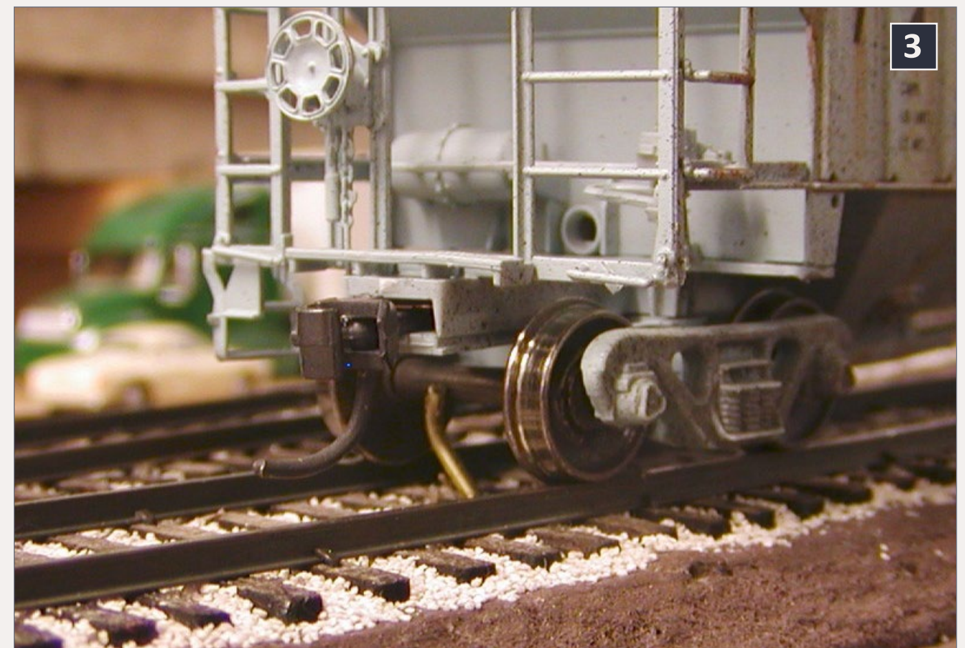
3: Joe Atkinson's brakes disengage automatically – the wire falls back in the hole when the car is pulled away. Joe Atkinson photo.
