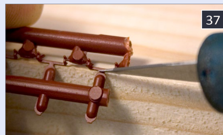
37: A block of wood under the sprue gate provides a solid surface for the cut.
