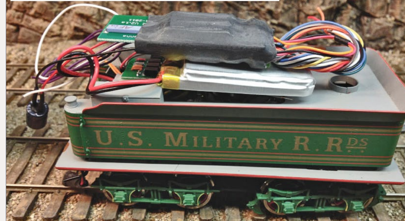
3: The "rat's nest" that confronted me when planning the installation of the Stanton Battery system. I had previously installed a QSI sound decoder in this loco. It had to be removed to accommodate the Tsunami decoder. I was able to use the same speaker.
