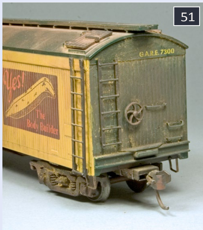
50-51: These two photos show an Athearn 50-foot express reefers which were upgraded using ladders and grabs. The dairy car on the left shows the original detailing. The dairy car is the same as the improved fruit reefer, but with a different paint scheme.
