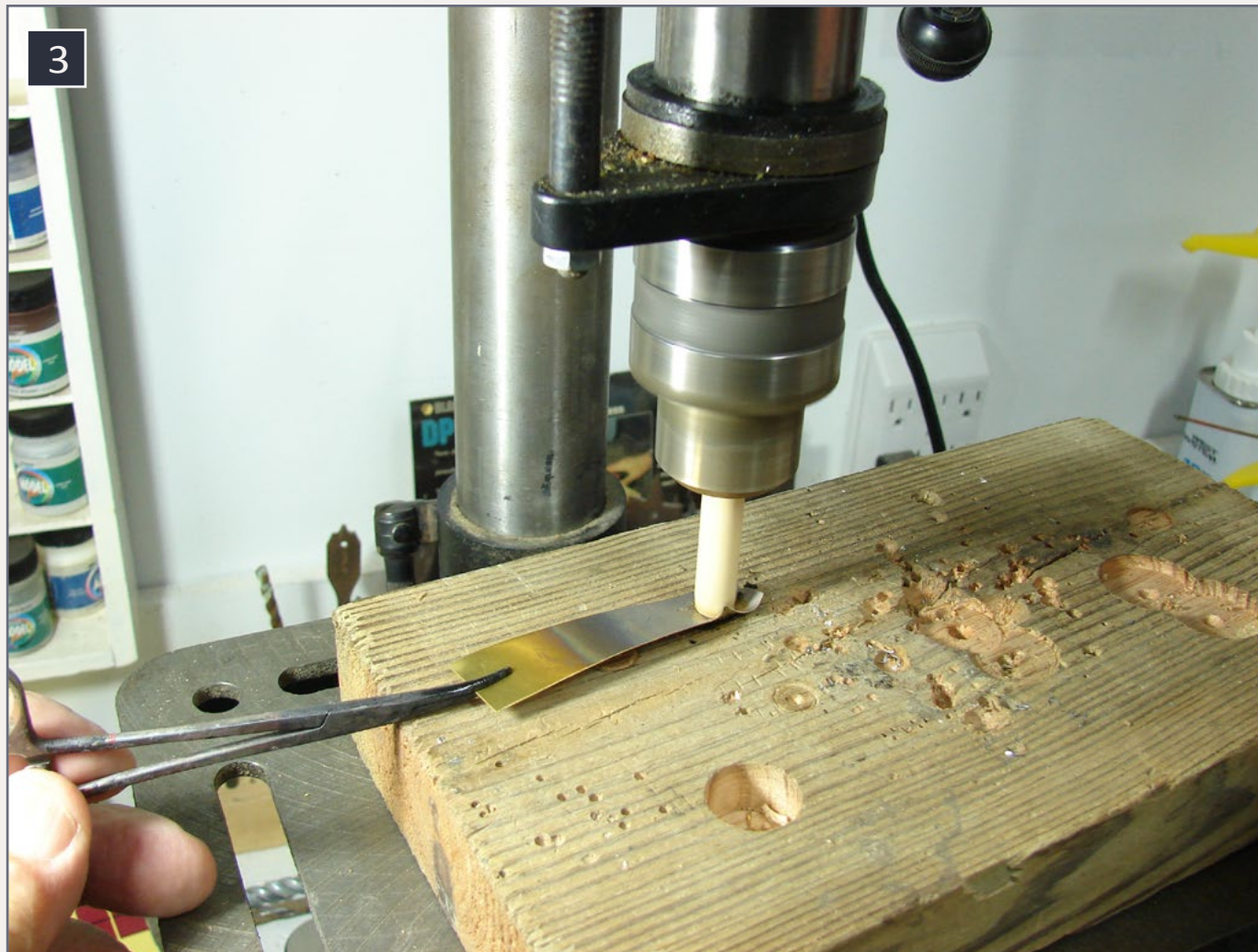
3. The reflector is formed by forcing a slowly-turning dowel into the annealed brass plate.
