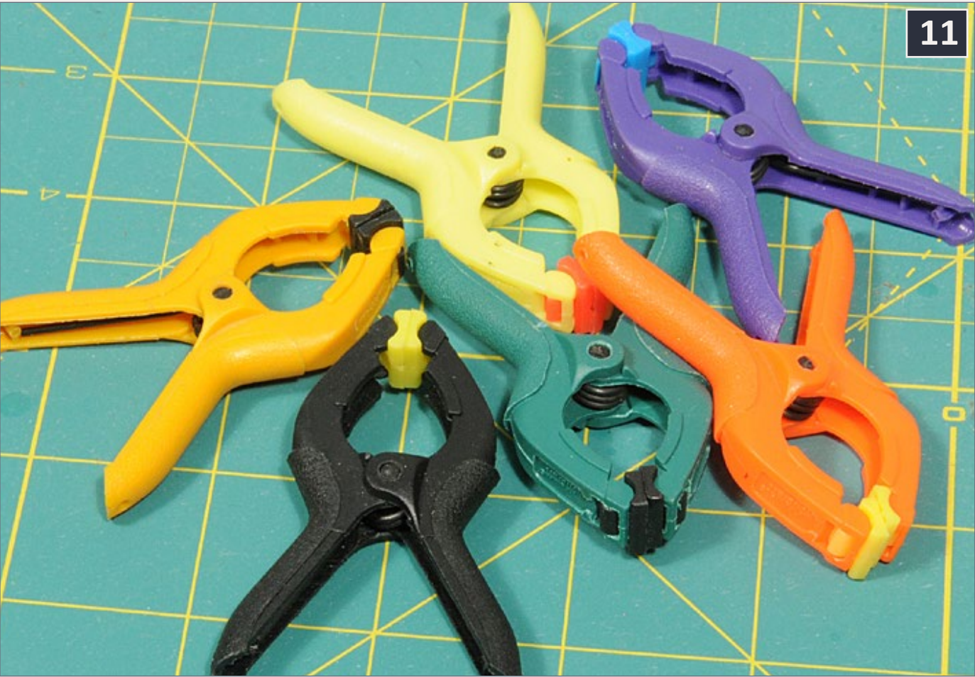
11: Spring clamps like these are available from Micro-Mark as well as some hardware stores.
