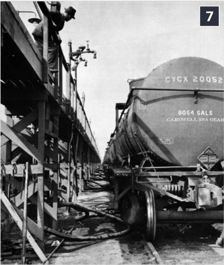
7: I Tank car unloading hoses at Standard Oil’s plant in Bayway, New Jersey. The platform above is for car loading. –Standard Oil Company photo, Rob Evans collection.
