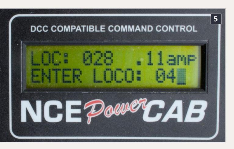
5: Programming the loco from figure 1 into an NCE Power-Cab with a long address of 04.
