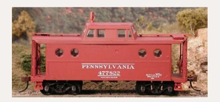
Bowser (bowser-trains. com) has a kit for an HO scale class N-5a steel cabin car with port hole windows. The model is
