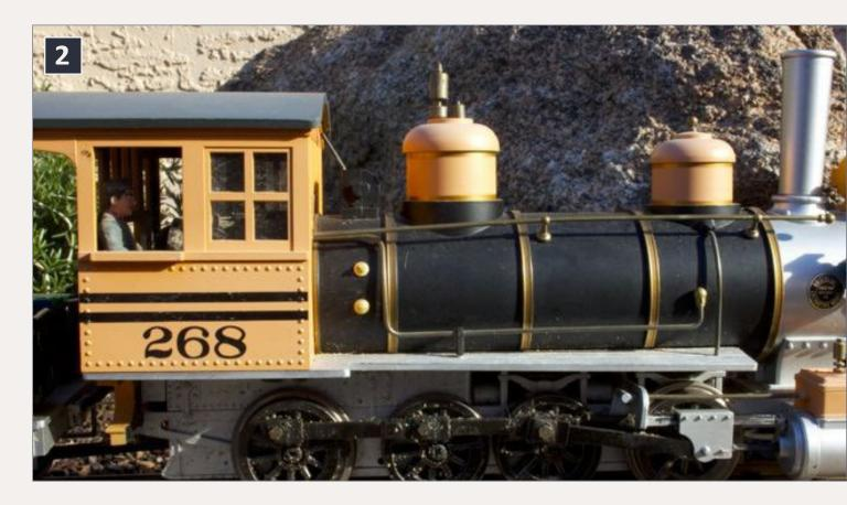
2: Loco with cab address of 268 – this will be a long address on any system, even though it has only 3 digits.
