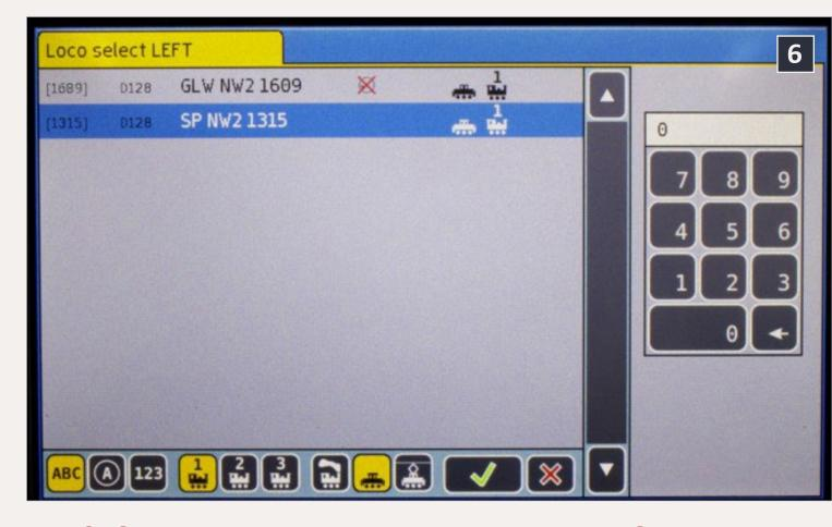
6: ECoS system loco selection pane, calling up SP NW2 1315 on address DCC address 1315.
