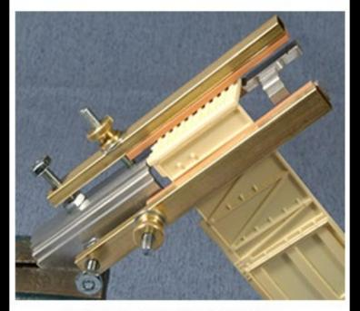
Combo Right Clamp TM with cast resin boxcar
