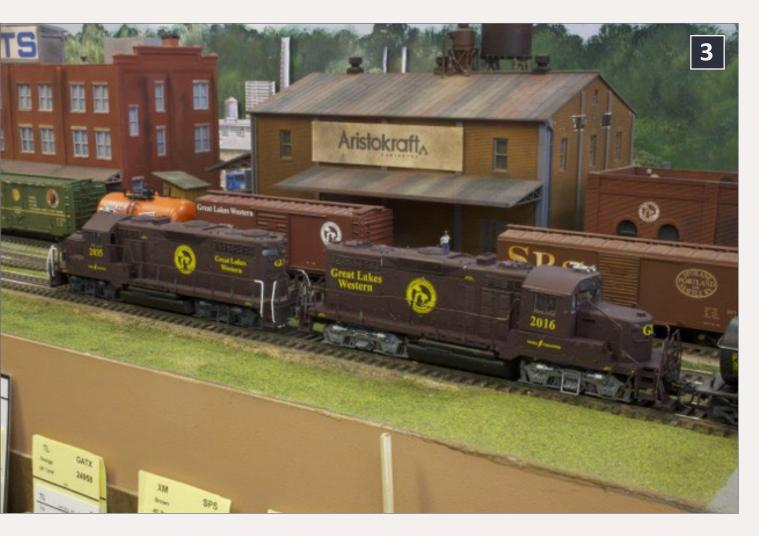
3: Two diesel locos making up a consist – this is train 103 from the PCMRC layout after it has run around its train and is ready to run back home. Loco 2016 has a value of 103 in CV 19; the 2035 has 231 (103 + 128) in CV 19. See figure 7.
