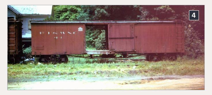
4: Tweetsie off-center door boxcar. Speculation has it that the cars were sized up from 28' cars, leaving the door where the center of the car would have been. Johnny Graybeal collection.
