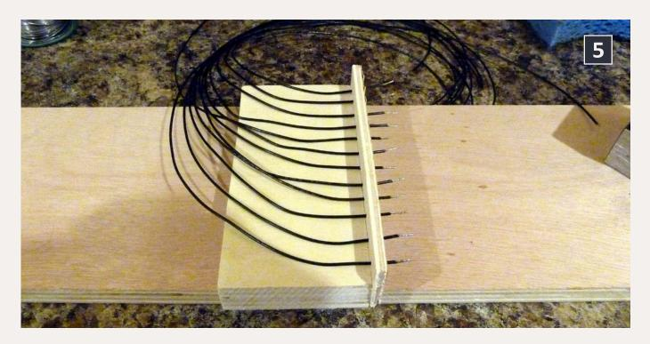
5: This a simple jig from scrap wood holds feeder wires to be tinned.
