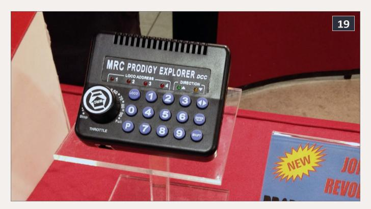
22: MRC announced their new Prodigy Explorer system, a starter DCC system for just over \$100 retail. Using their handheld throttles, this system is expandable.
