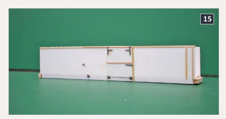
15: The 36' car attached to the underframe. Note the end sills are not yet filed even with the car sides. They also need a metal corner plate attached to them.
