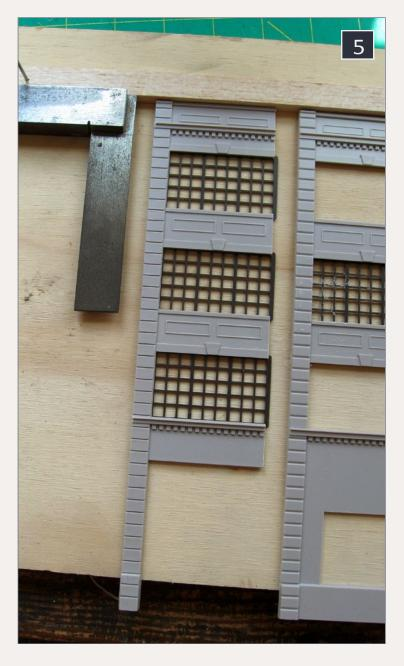
5: A homemade jig will keep things square as you cement the wall to the rest. Don't cement the windows in, but place them in the opening to make sure they'll all fit later.
