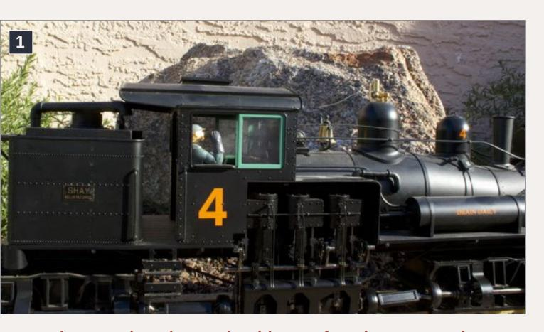
1: Loco with a short cab address of 4 – I run it as a long address on NCE by programming it as a long address and selecting it as 04.
