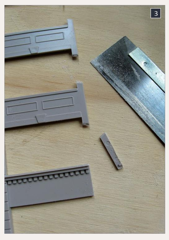
3: Then cut it flush to the windows, using a razor saw.
