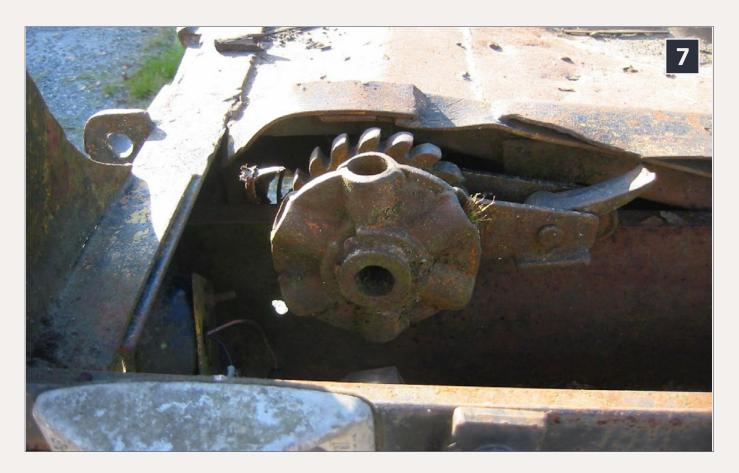
7: Here is detail of the ratchet system that is used to tie down the autos during transport.
