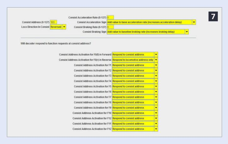
7: DecoderPro screen shot – setting up CVs 19, 21 & 22 within the Consist panel – loco # from the PCMRC layout.
