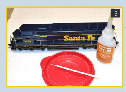
Brush to apply CA where the metal stanchion plugs into the plastic body. I squeeze the CA into a plastic KFC side order lid and dip the Micro Brush in that. That solves the movement problem.
