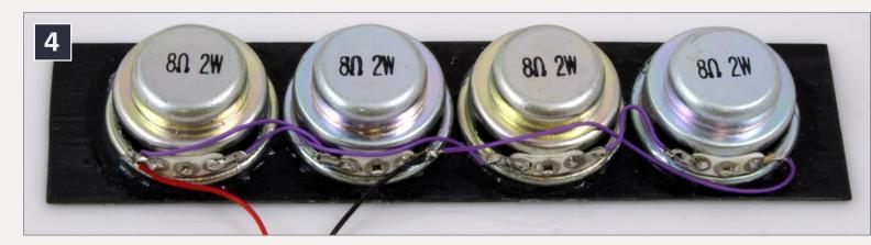
4: Line array of four identical speakers - wired in a seriesparallel combination, the resulting unit is rated at 8 ohms and 8 watts.
