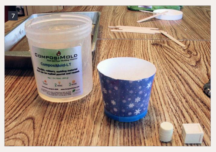
7. The mold box for an O scale barrel and crate consists of a cut-down paper cup.
