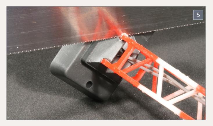
5: The final step in tearing it down is to remove the crude oversize base from the lattice tower by carefully cutting through each leg with a razor saw.
