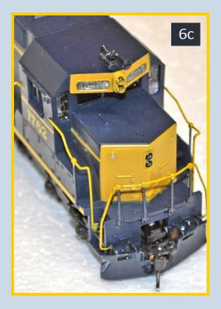
6c: I paint the plow Santa Fe blue. While working on the ends, I paint the running lights with a touch of silver to represent the clear glass lens.
