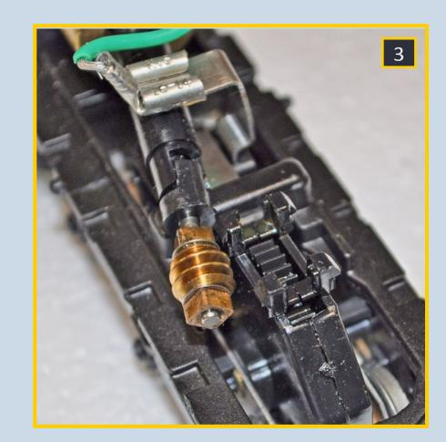
3: Remember the Athearn "growl"? You can tone this down. Carefully pry off the gearbox cover on each truck. I have used Vaseline for years with no problems for this step. If you are not comfortable using Vaseline, apply a plastic-compatible grease to all of the gears you can see. Put in a large amount. Apply it to the metal drive gear also. Put the unit on your track and run it back and forth a few times to work the grease through the gear system. Apply more if unit continues to growl.
