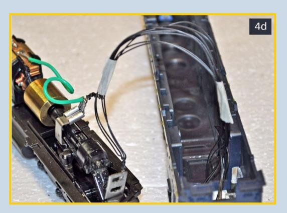
4d: Solder the + wires to the power clip, and the – wires to the metal clip on the power chassis for the negative ground. Tape the wires together to ensure they don't foul the gearing and the motor. Reattach the shell to the power chassis.
