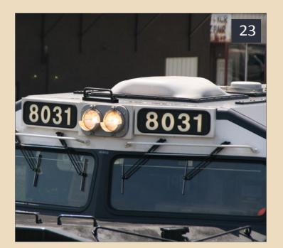
23: This Norfolk Southern locomotive shows us the large square dome style that incorporates multiple antenna technologies into one protected unit.
