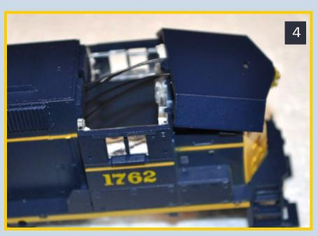
4: Attach the light bulb wire to the terminals and solder it to the positive wire on the motor as shown. The terminals slide onto the truck clips.
