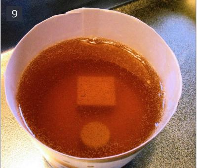
8. The masters are stuck to the bottom of the cup with hot glue before pouring heated ComposiMold.
