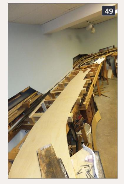
49: Once I'd arrived at a track layout, I used the track arrangement to mark the cuts on the big sheet of plywood, and the here is the result. Note the cut at the bottom to fit existing sub-roadbed.
