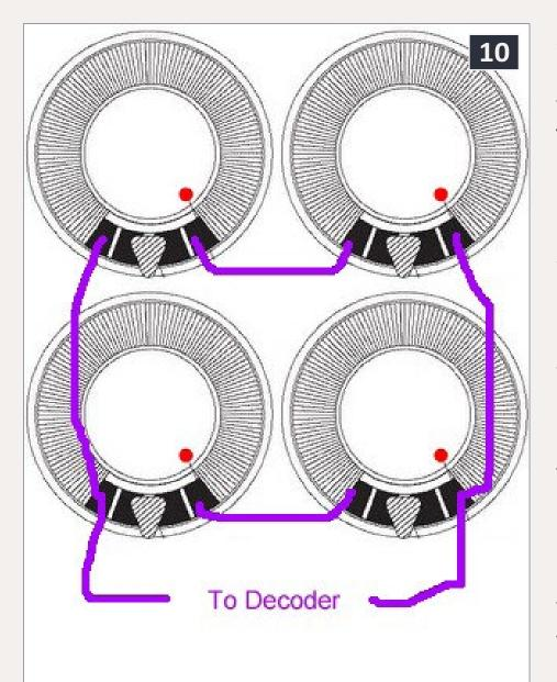
10: Four speakers in a series-parallel array – the final impedance will be the same as the speaker impedance – 8-ohm speakers will yield an 8-ohm load.
