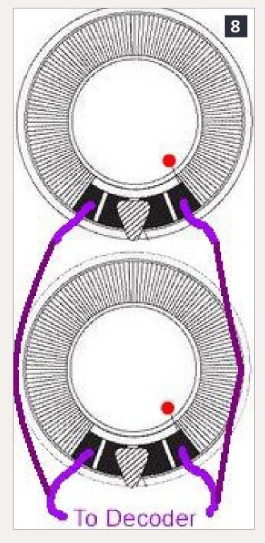
8: Two speakers wired in parallel – the final impedance will be half the speaker rating – 8-ohm speakers yield a 4-ohm load.
