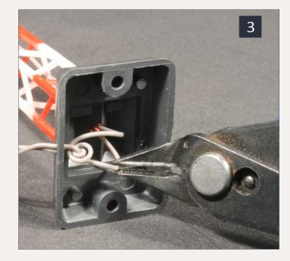
3: Begin disassembly of the microwave tower by cutting the wires at the base.
