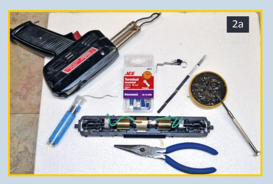
2a: Here are the tools I use, along with the discarded parts. From left to right: a solder gun, solder, insulated terminals, pliers, soldering paste, jewelers flat head screwdriver, and some wire to reconnect the power from the motor to the trucks.
