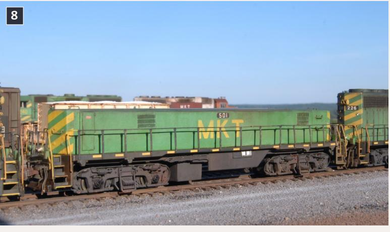
8: His custom-built slug uses an Atlas frame and trucks. The body is built from styrene and painted with Modelflex. Added details include MU cables, actuating hoses, sand lines, traction motor cables, and oil and pastel powder weathering.
