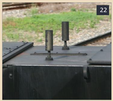
21: The roof of this Norfolk Southern locomotive provides a clear contrast between the Sinclair style and the smaller EOT antennas. Multiple antennas often indicate the locomotive is equipped with additional specialized radio equipment for features such as DPU (mid-train helper) control, allowing the additional units to be operated from the lead locomotive.
