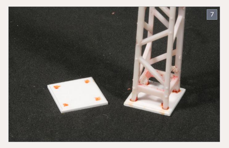
7: Dip the legs into a stamp pad. Carefully place the tower on the base, allowing the bottom tip of each leg to transfer the stamp ink to the base, instantly creating accurate points that can be drilled with a pin vise.
