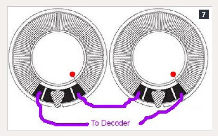
7: Two speakers wired in series – the final impedance will be twice the speaker rating – 8-ohm speakers yield a 16ohm load or 4-ohm speakers yield an 8-ohm load.
