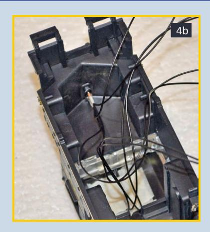
4c: I use Miniatronics Corp. incandescent 12 volt 30mA 1.7mm diameter lamps. I had to slightly ream the existing holes to accommodate the lights. 4b: Cement them in place with CA. I use masking tape to hold the top lights in place before gluing them.
