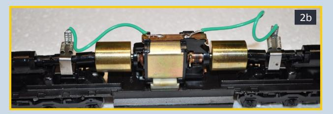
2b: I attach the wire to the terminals and solder the wire to the positive wire on the motor as shown in the picture. The terminals slide onto the truck clips. The negative connection is made by the metal clip on the motor bottom that contacts a polished spot on the frame.
