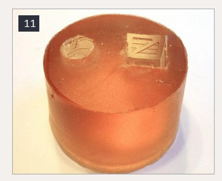
11. The cured **ComposiMold flexes** enough to release this master easily. The detail from the crate can be seen in this picture of the mold.
