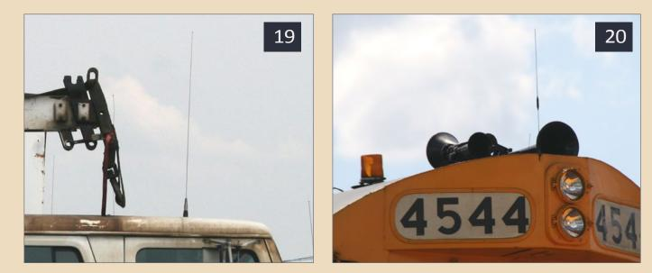
19-20: The roofs of this maintenance truck and a locomotive show two installations of whip antennas. Whips are generally mounted near the center of a roof to create a ground plane which optimizes the performance of the antenna.
