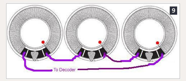
9: Three speakers wired in series – the final impedance will be three times the speaker rating – 4-ohm speakers yield a 12-ohm load.
