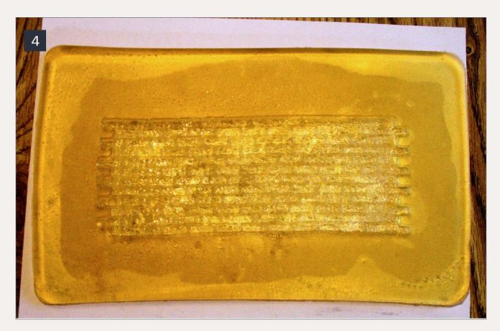
4. The wall section mold produced by ComposiMold.
