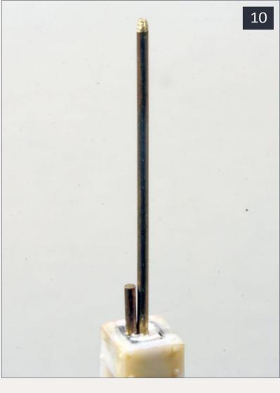
10: With both the antenna and support pipe extending upward from the tower, we can now fashion brackets from styrene strip to tie them together.
