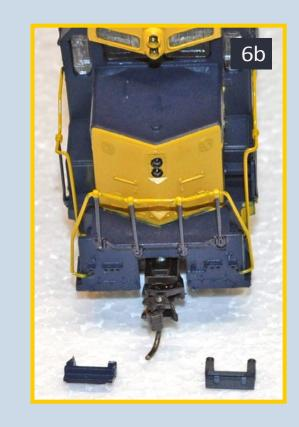
6-6a: Apply the air brake cylinders supplied by Athearn. Although I am not super detailing the model, I did replace the original air-horn set with a more prototypical one, a Details West AH-190 Leslie RSL-3L-3R. This small addition makes a big difference.
