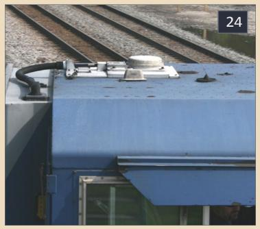
24: This array on the roof of a CSX locomotive shows us a variety of antennas, including a small whip, a wide cone, and a small dome style. ■
