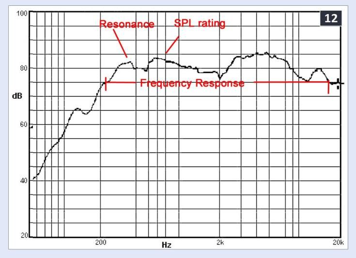
12: Frequency response (sound pressure level or SPL vs. frequency) of a typical speaker used in model railroading (28 x 35 mm – 8 ohms).
