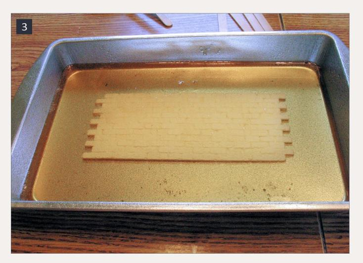
3. ComposiMold as poured, with room left around the master to produce a stable mold.
