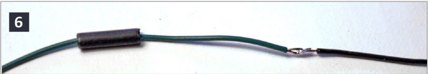
6: Soldered splice, ready for shrink tubing.
