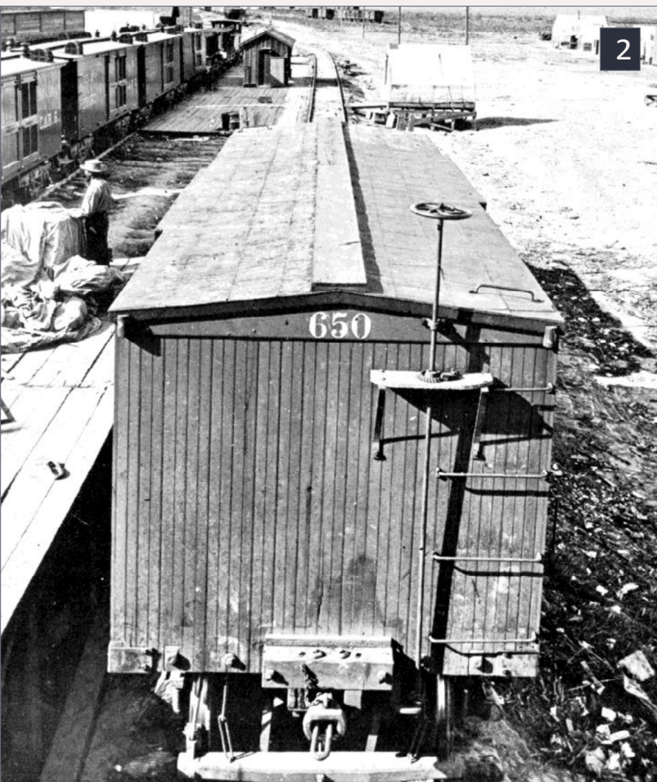
2. Vertical "stem-winder" hand brake from 1869.
