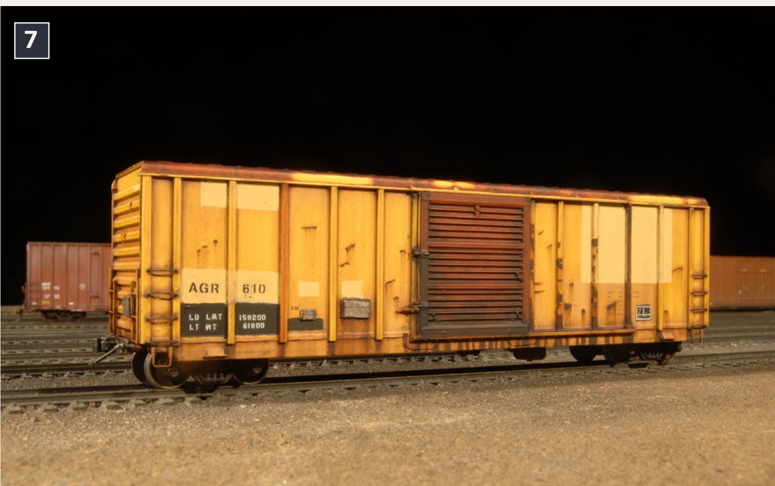
7: The AGR box car (Athearn) is loosely based off the prototype. He added Details West air hoses and used balsa wood for the tack boards. All weathering done with artists oil paints.
