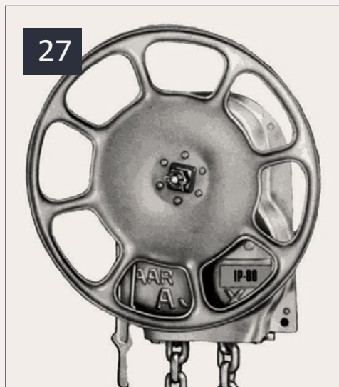
27. Ajax model IP80 with release lever at the lower left.
