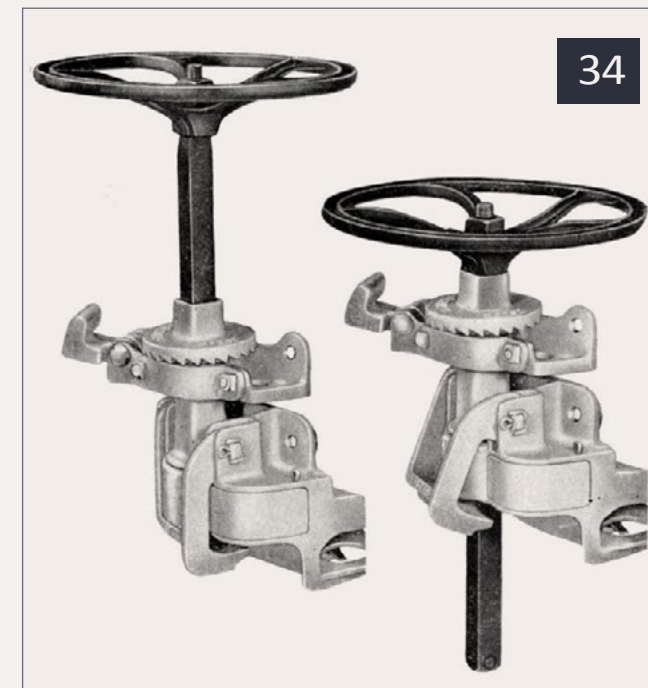
34. Universal geared drop-shaft hand brakes in use since the 1970s.
