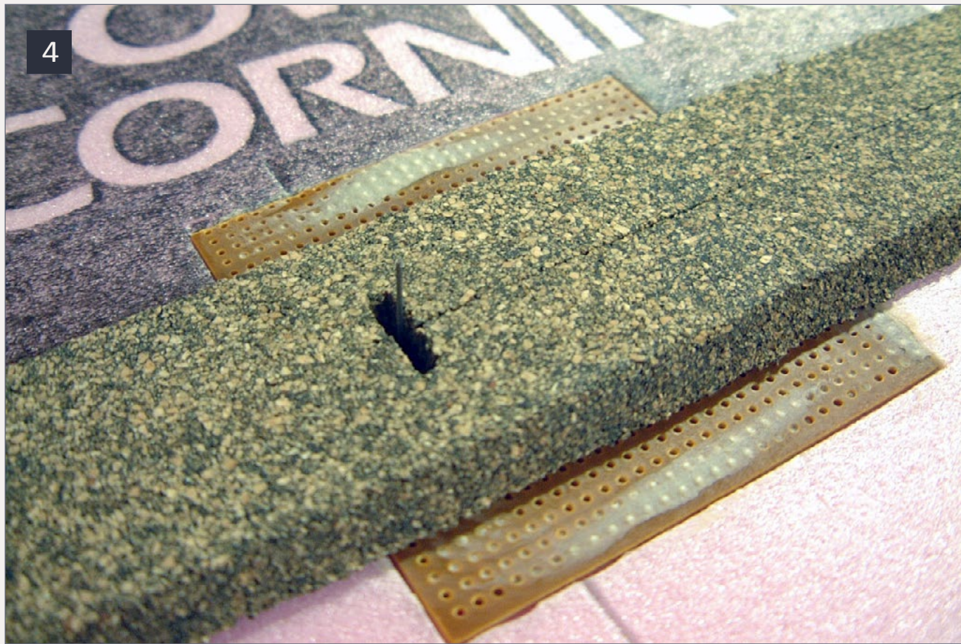
4: Glue is applied and switch machine installed. A slot is cut into the cork roadbed for the actuator wire.
