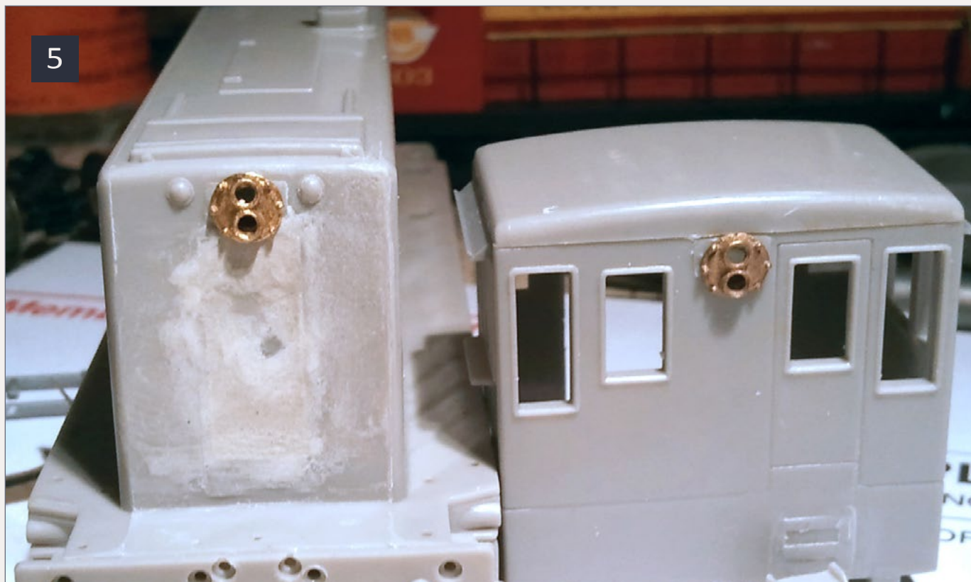
5: Cal-Scale headlights have been added to the cab and hood. The cab steps have also been removed to allow decaling of the diagonal stripes on the back of the cab.
