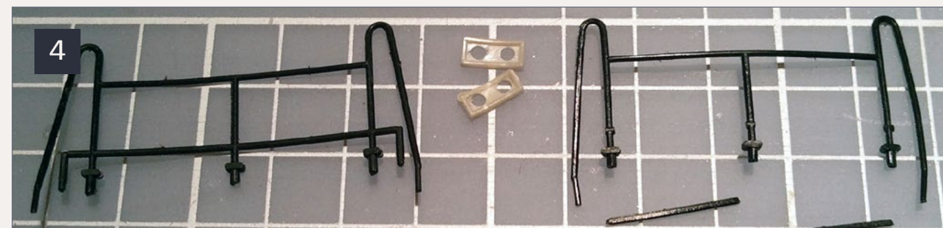
4: The kit supplied handrail is on the left, compare this to the modifications on the right. The headlight castings are in between the handrails. They will be glued to the side of the locomotive to become the number boards.
