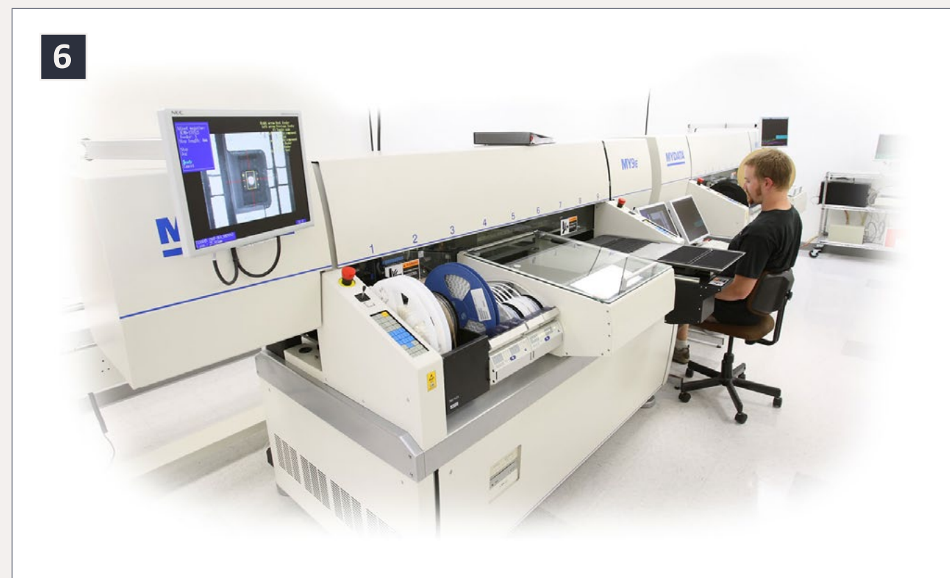
6: One of SoundTraxx' two pick-and-place SMT assembly machines – keeping the jobs and technology in the U.S.A.
