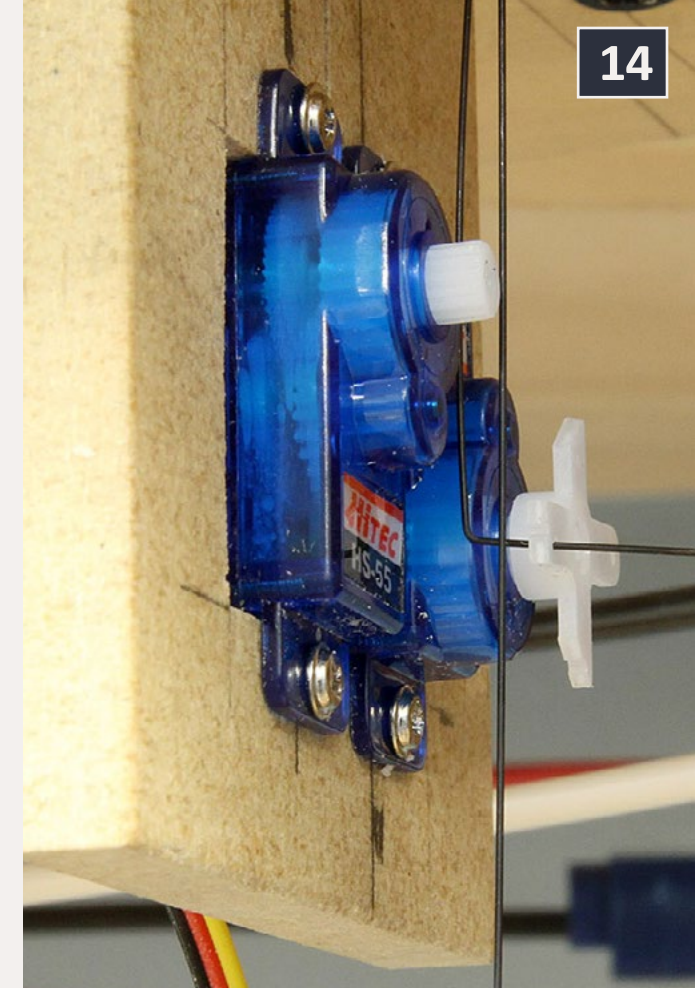
13: Threading the servo control arm onto the bent semaphore control wire.
