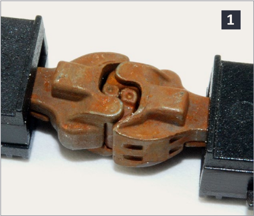
1: Sergeant HO scale couplers function like the prototype, with a ball dropping in place behind the knuckle arm to lock couplers closed. Graphite lubrication and careful removal of casting flash is vital to smooth operation.
