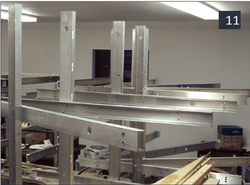
11: This is the framework at east end of Norton Yard on the upper level. On several of the horizontal pieces you can see my markings for the location of the channel along with the length I need for the channel.
