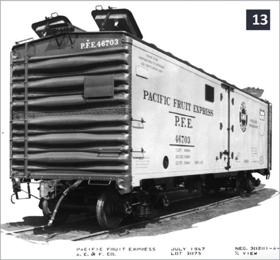
13: This builder’s photo of a Class R-40-23 car with ice hatches latched open clearly shows the one-piece design of plug and cover, along with the latching hook underneath the plug which permitted locking hatches from inside (mostly to prevent transients from riding in empty cars). – American Car & Foundry Company photo for PFE, courtesy CSRM.
