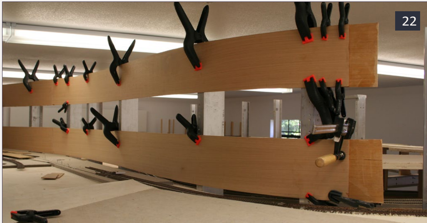
22: I am beginning backdrop construction. The plywood strips will help provide additional support and stability.
