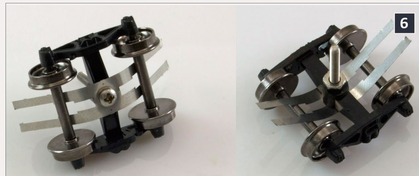
6: Richmond Controls wiper kit and Intermountain wheels on an HO scale truck
