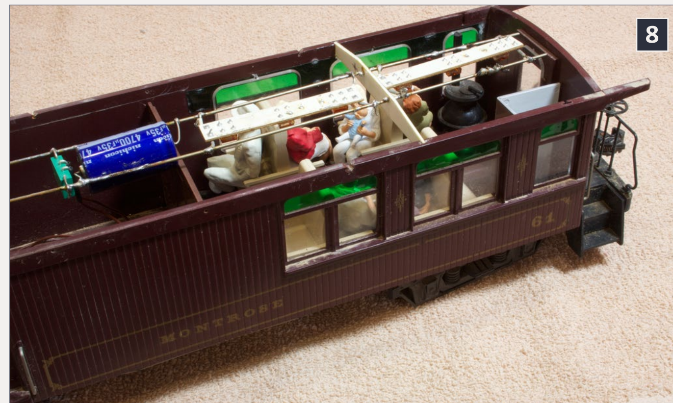
8: Lighted passenger car from figure 1 with the roof off, showing LED packages installed
