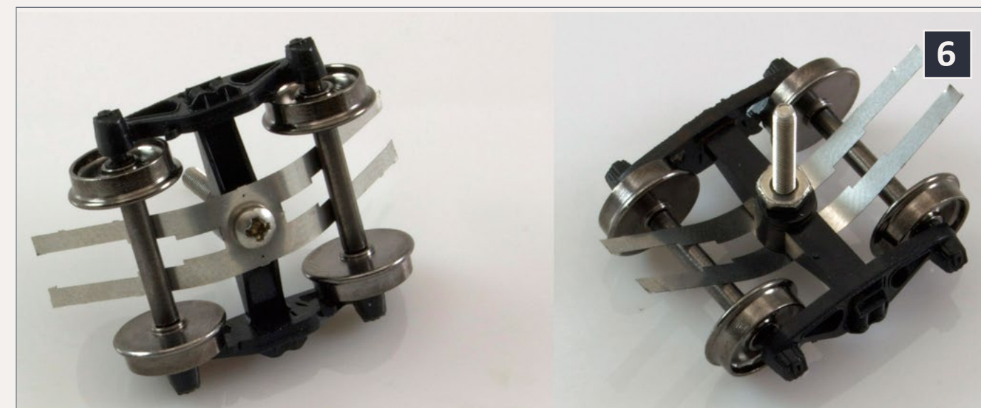
6: Richmond Controls wiper kit and Intermountain wheels on an HO scale truck
