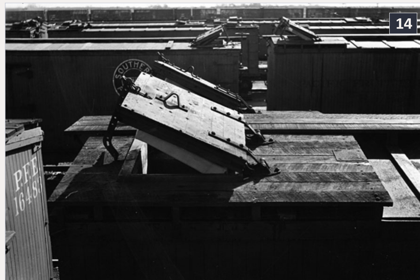
14: This ice hatch is latched as far open as it can go (note top of latch bar), for ventilation service. The hatch plug underneath is separately hinged, thus is at a slightly different angle. – PFE photo, courtesy CSRM.
