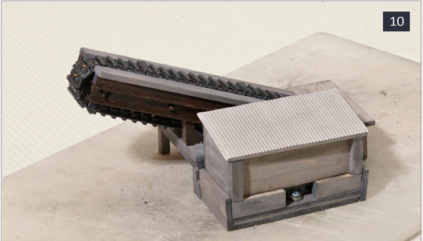
10: The other side of the conveyor shows the structure that I used to house the motor and gear set.
