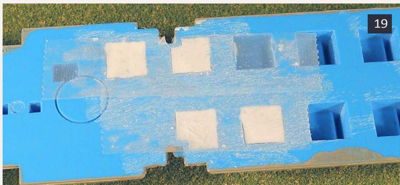
19: The underside of the Camellia. The cavities of the four seats to be removed have been filled in with putty.
