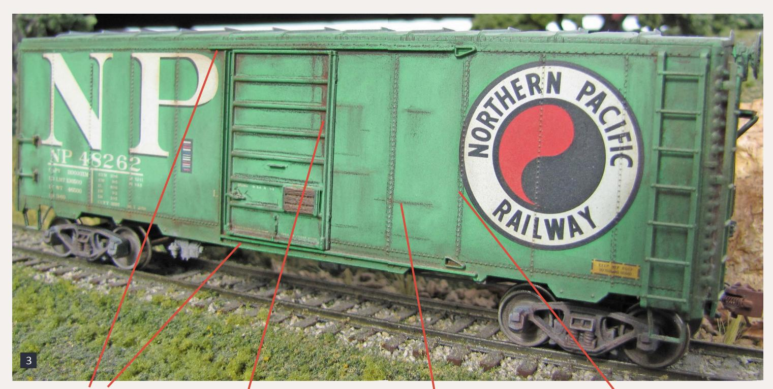
Use pencil along door tracks to add dirt buildup Use pencil along door ribs to add accumulated grime and rust Use pencil to add rust streaks from door scrapes
