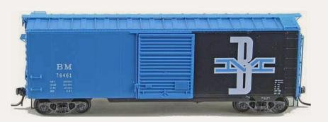
scheme. Both models will be fitted with Kadee two-piece self-centering trucks and #2100 couplers.
