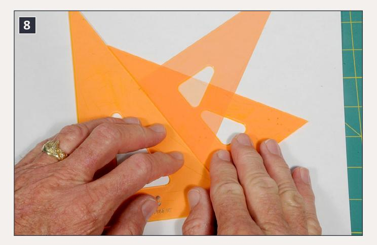
8: By turning the "sliding" triangle 90°, as shown by the "ghost image", you can easily draw or cut something at a 90° angle to the base line. The 90° angle is formed in the space between the two triangles directly above the middle finger of my right hand.
