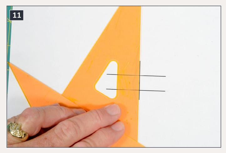
11: The sliding triangle is then turned to result in lines at 90° from the initial lines. Here the sliding triangle is aligned with the pencil mark for the right edge of the window opening.
