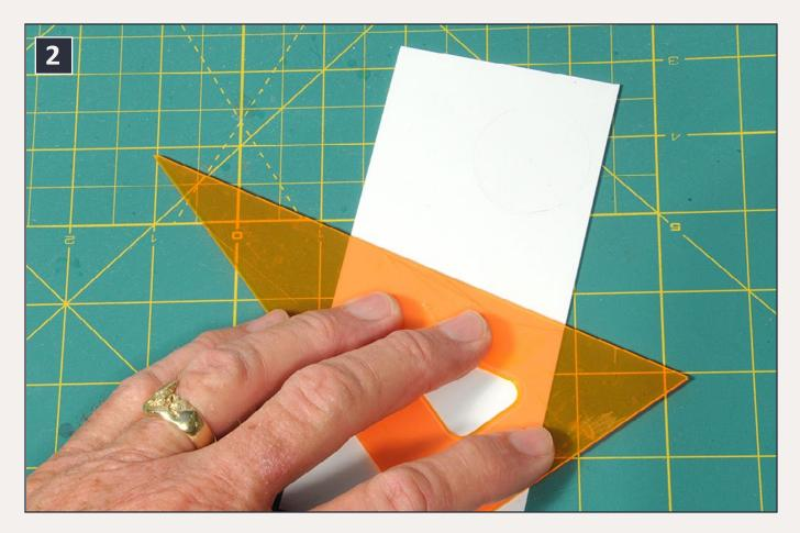
2: It is much easier to hold a triangle than a narrow scale ruler, as shown here. This makes it easy to ensure that the straightedge doesn't move as you are cutting a piece of material.
