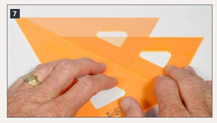
7: When you have two drafting triangles, you can easily make parallel lines. The fixed triangle is on the left (since I am lefthanded) while the sliding triangle is on the right. Here I am moving the sliding triangle upwards while holding it against the fixed triangle to create two parallel lines. The "ghost image" shows the sliding triangle after being slid toward the top of the photo.
