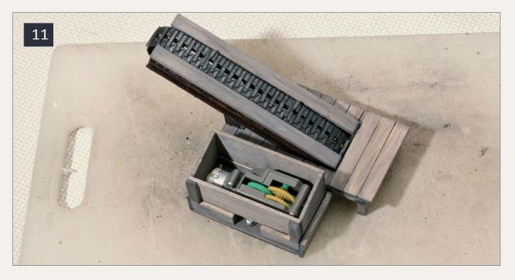
11: I have removed the roof to expose the motor and gears allowing me access for maintenance that might be needed. This provides a good view of the fit inside.
