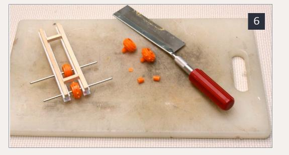
bass that I attached to the H beams to maintain the proper spacing. You can also see the extensions that are trimmed from each of the Tamiya wheels.
