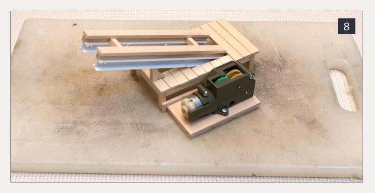
8: A wood pad was used to mount the motor and connect it to the lower conveyor frame. I also added two strips of basswood to act as guides to keep the conveyor track in alignment.
