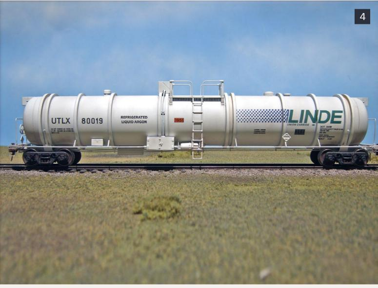
**4:** Robert Pitts built this unique model of UTLX 80019, a cryo car built in 1962. The cars were designed to haul 15,000+ gal of liquid argon at -302 degrees Fahrenheit This car falls into the general category called RailWhales. The construction of this type of car was ended by Federal regulations that went into effect in December 1970.
