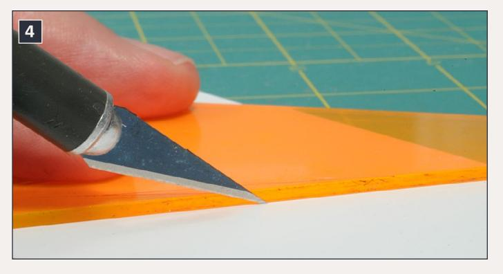
4: Holding a hobby knife at a shallow angle (along with the shape of the No. 11 blade) makes it easy to avoid cutting the drafting triangle itself.
