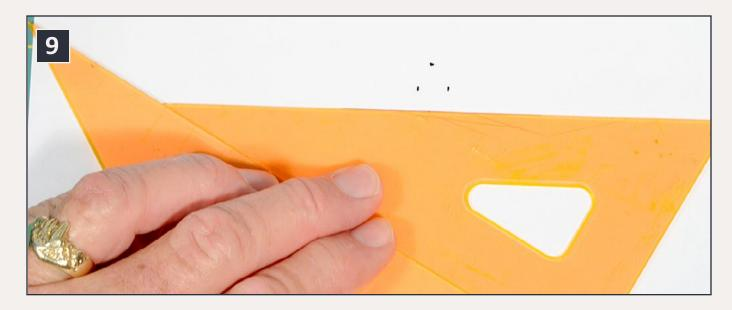
9: These four photos show how you can easily make a template for cutting a sheet of clear styrene to make window glass for a window casting. There are pencil marks on the paper for the horizontal and vertical extents of the window opening. In this view, the sliding triangle is aligned with the bottom pencil mark.
