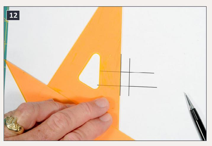
12: The sliding triangle is now slid to the left to be aligned with the pencil mark for the left edge of the window. The window template is now complete.
