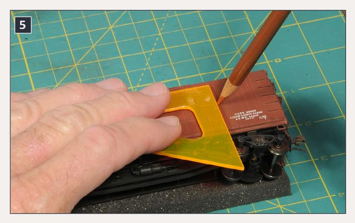
5: Here a small drafting triangle is lightly tucked up against the letterboard of this freight car so that a colored pencil can be streaked downward along the side of the car.
