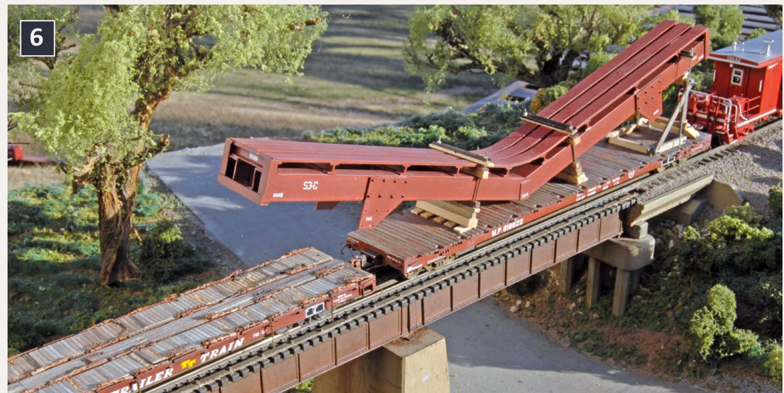
6: Dave's bridge beam load viewed from above. The idler car detail shows clearly. The load is blocked with wood fastened with steel, bolts, and nuts.
