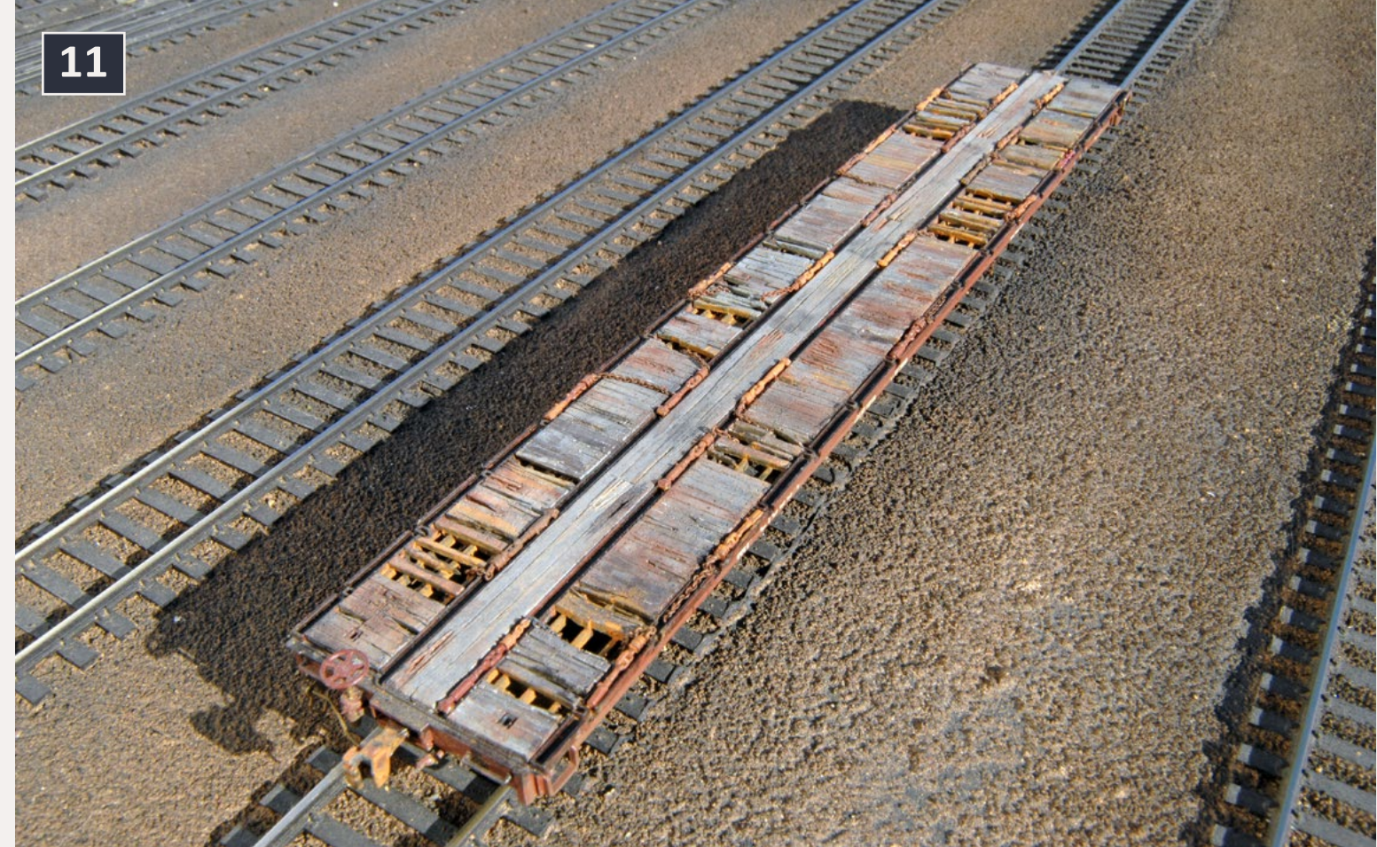
11: An InterMountain flat car has seen better days. The heavy weathering of the board by board deck was achieved with shades of gray lacquer paints. This car was inspired by Greg Moe in a RailModel Journal article in 2000.
