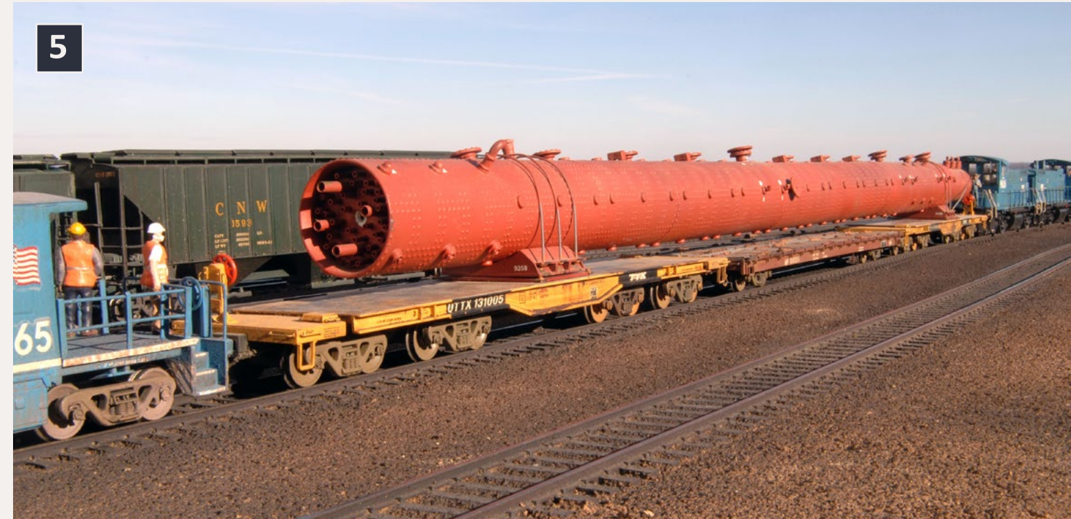
5: This small refinery fractionating tower is loaded on three flat cars. The outside flat cars bear the weight while the center idler flat keeps everything together during movements. The video shows the load running through a curve, illustrating the swing of the load and the cars in action.
