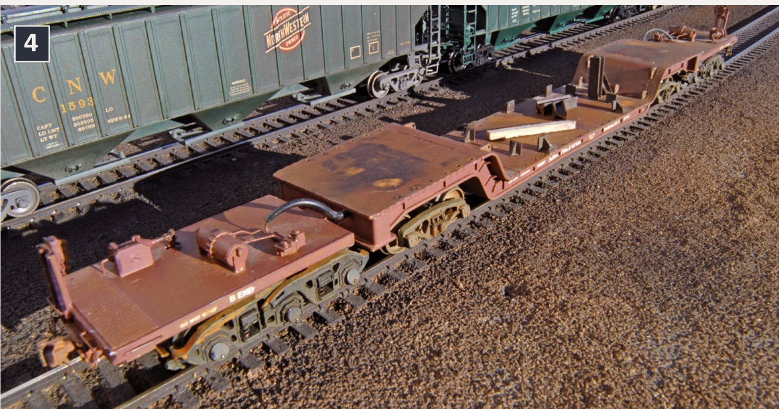
4: This model, representing a General Electric-style prototype, sports two Buckeye and two standard AAR 40-ton trucks. The model shows the flat car after the load has been removed, with some of the supporting steel brackets still in place.
