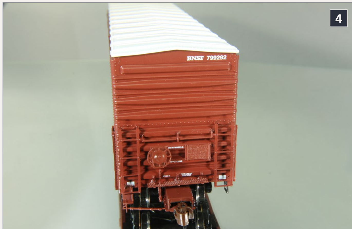
4: Brake wheel end details.
