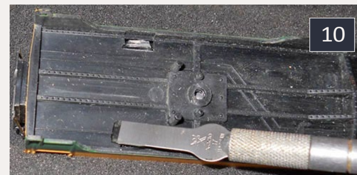
10: Next I remove the ridges along the edge of the body.
