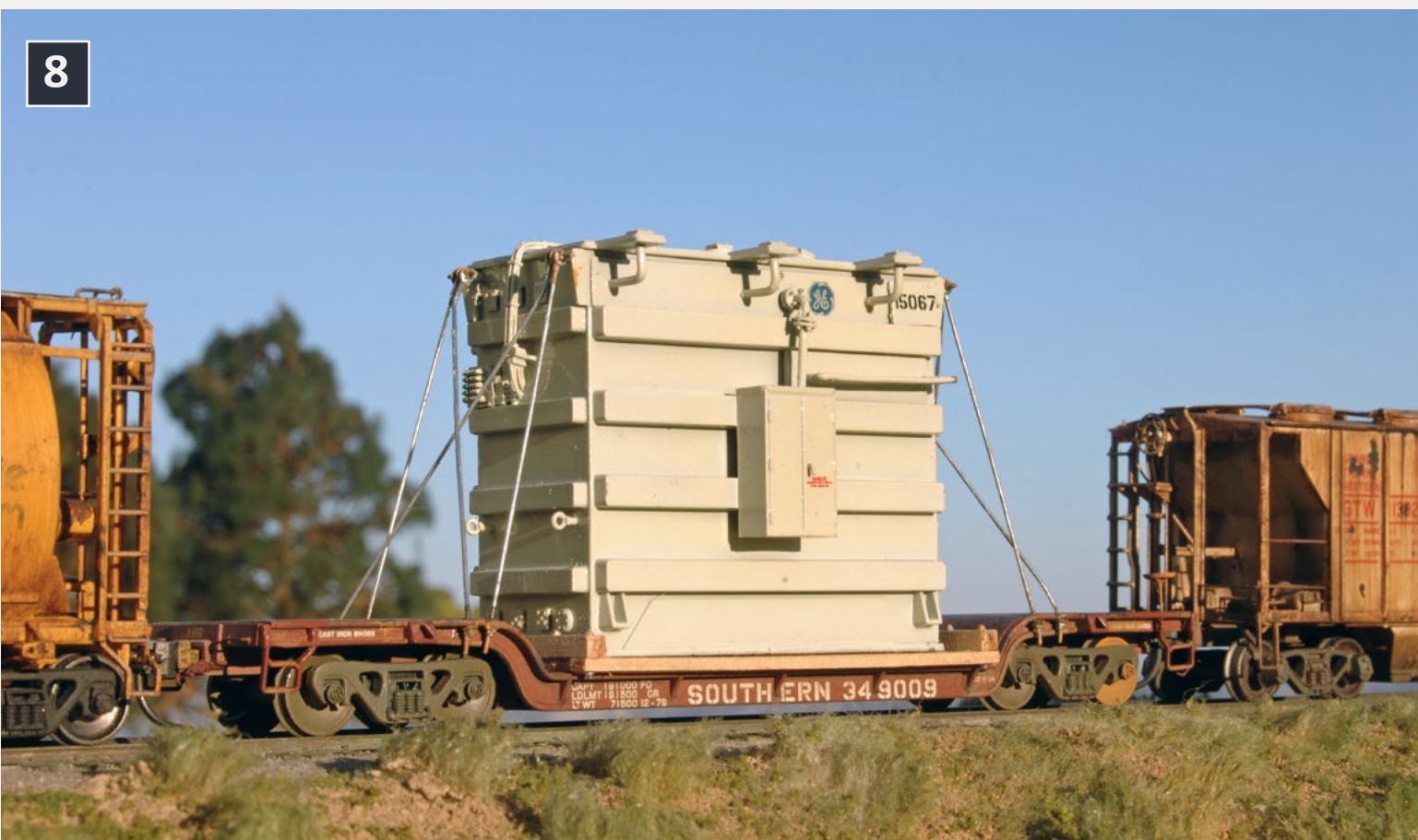
8: The Walthers transformer is loaded on a Walthers depressed-center flat car with Athearn 100-ton trucks and Sergent scale couplers.
