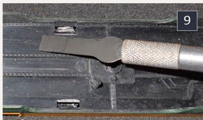
9: I began removing the air line for the new body mount coupler kit.
