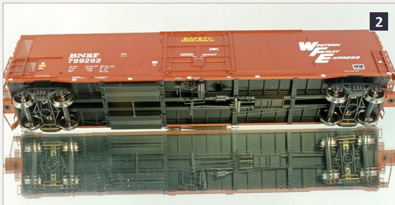
2: Underframe and brake details.
