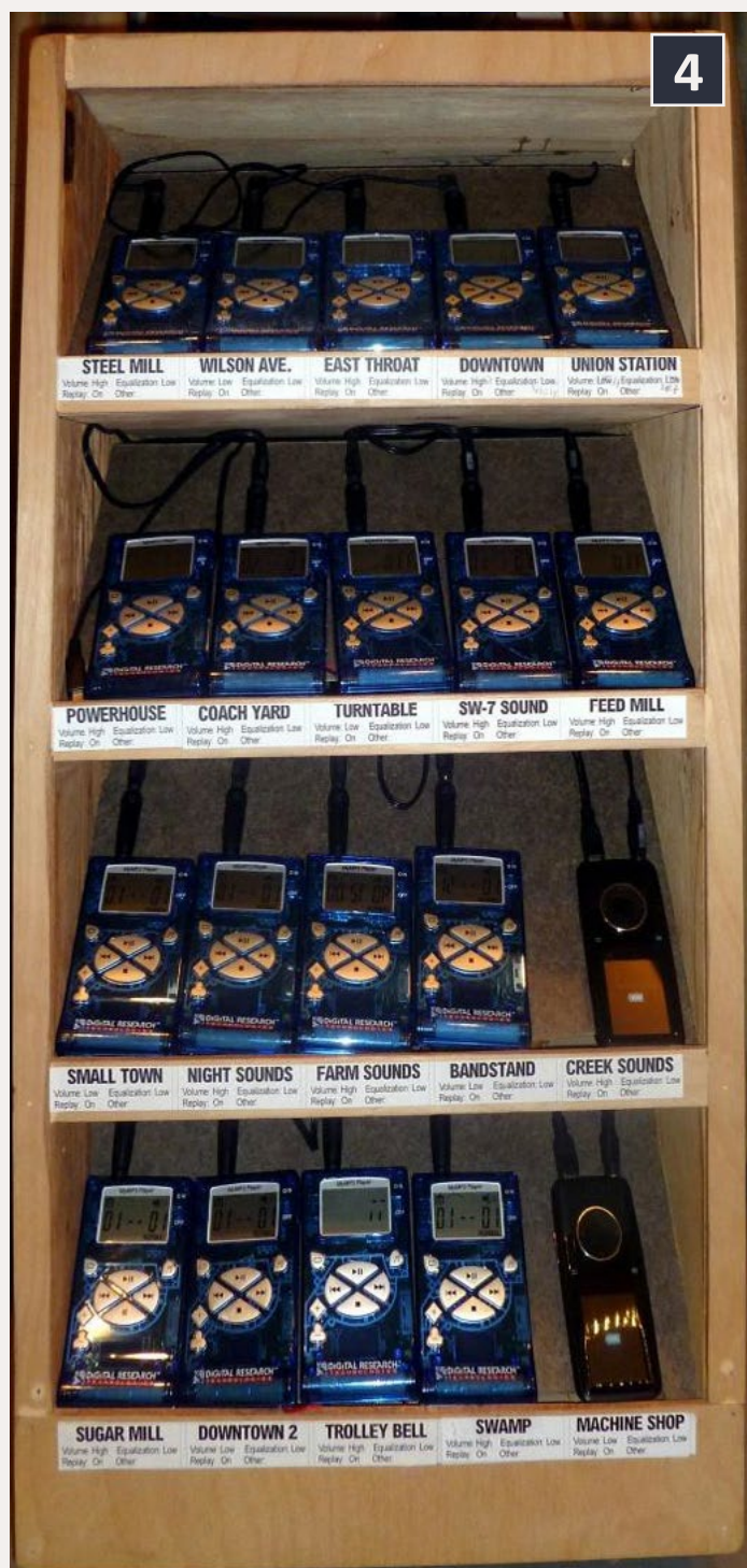
4: This is a front view of the component cabinet with each MP3 player labeled for its appropriate sound track.
