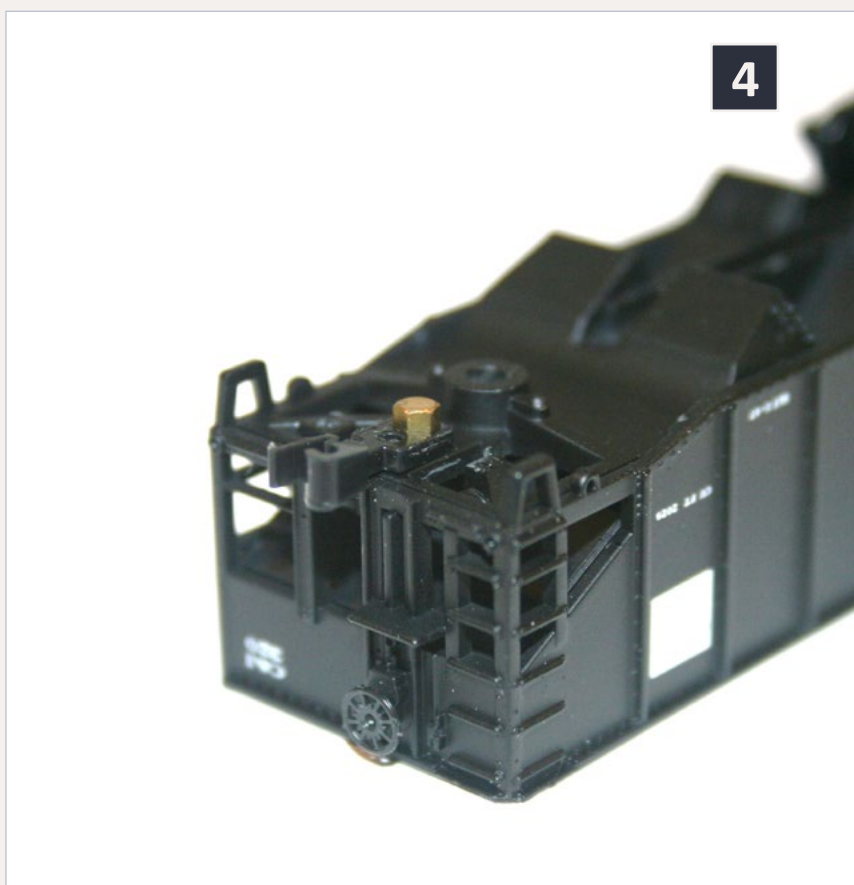
4: AccuMate (Red Caboose) non-operating couplers applied to a two-bay hopper.
