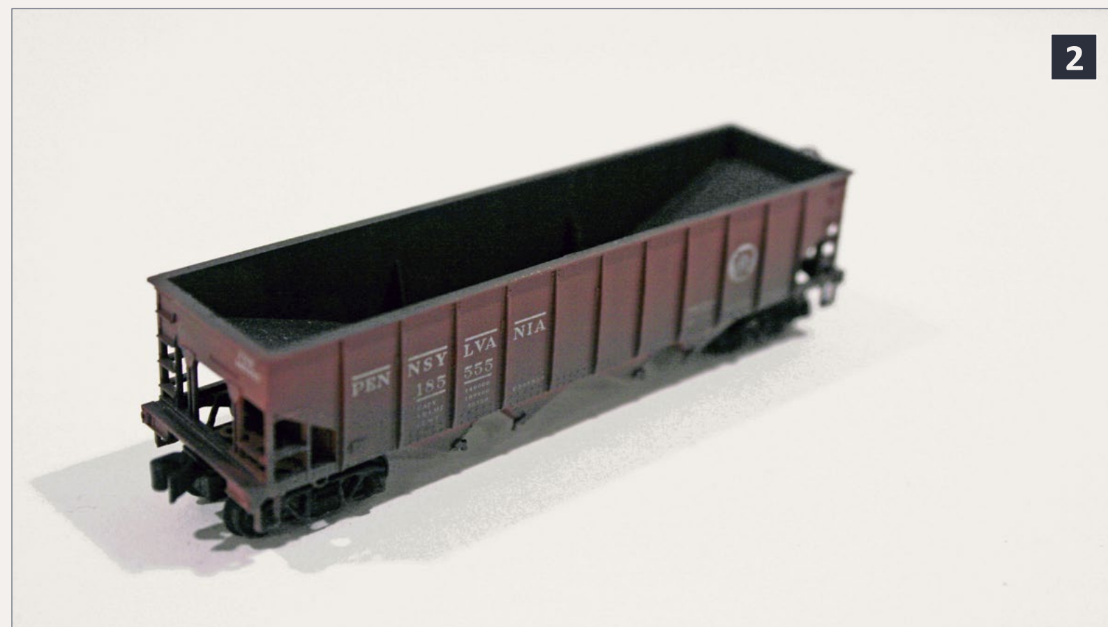
2: Bowser slope sheet weight applied to a four-bay hopper. A little weathering makes the weight almost invisible.
