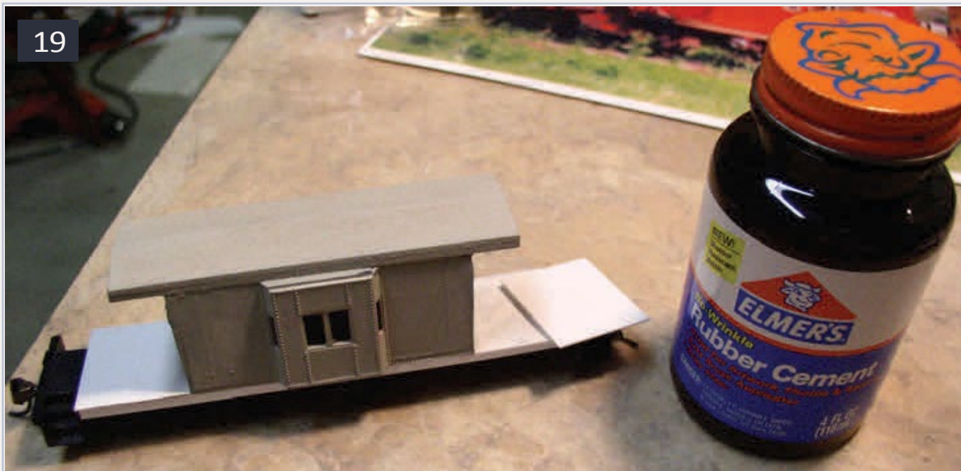
19: Add thin styrene decking to the ends. To stop the plastic from melting, I glue the porches down with Elmer's Rubber Cement instead of plastic solvent cement.
