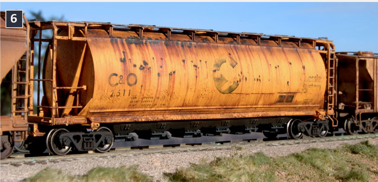
6: Joe used a sandblaster to show the effects of sun and wind on this Atlas cylindrical hopper, then added rust effects using oil paints.
