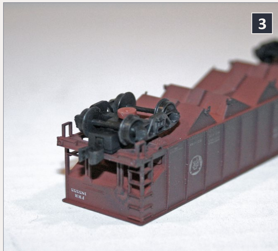
3: AccuMate (Red Caboose) T-shank couplers fit easily into the Bowser trucks.
