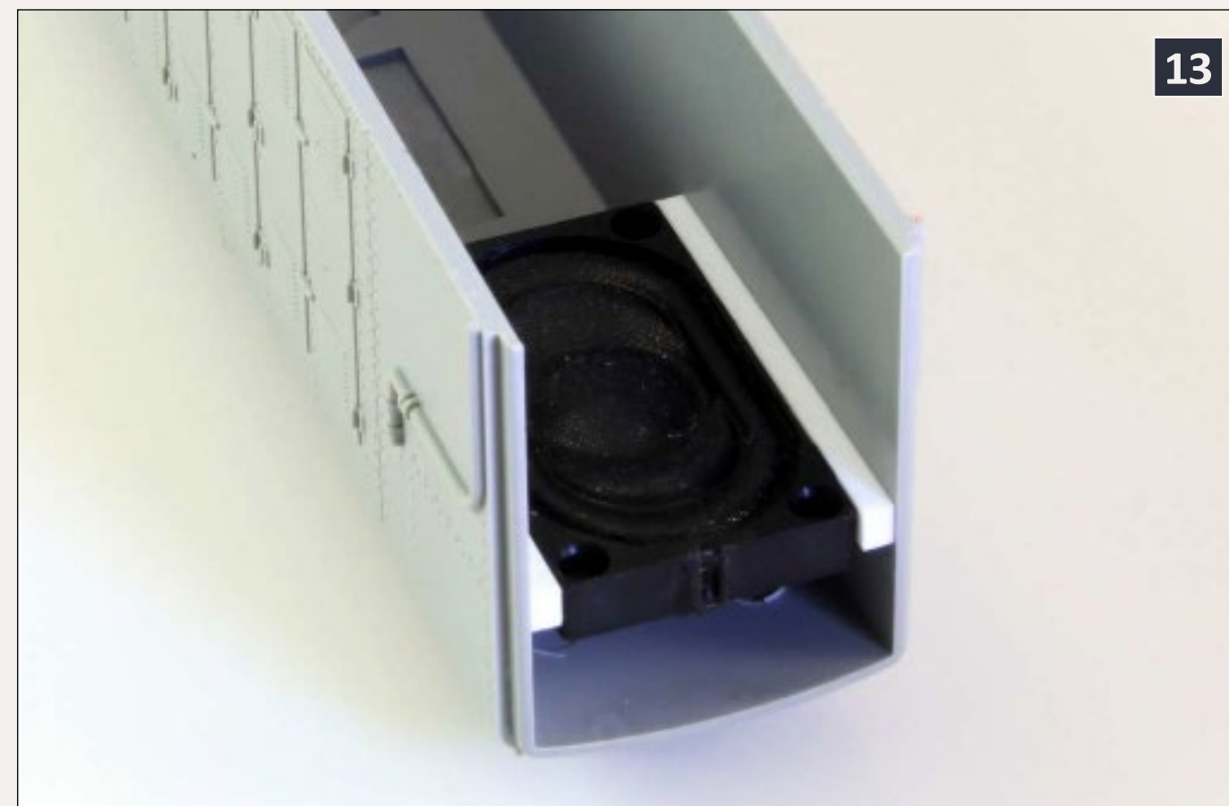
13: The speaker is cemented into shell of the Atlas S-2.
