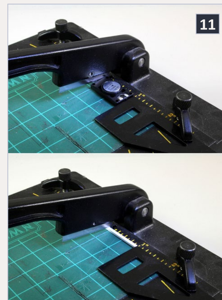
11: To measure the length of styrene needed to match the speaker I simply use the speaker as a guide to set the stops.
