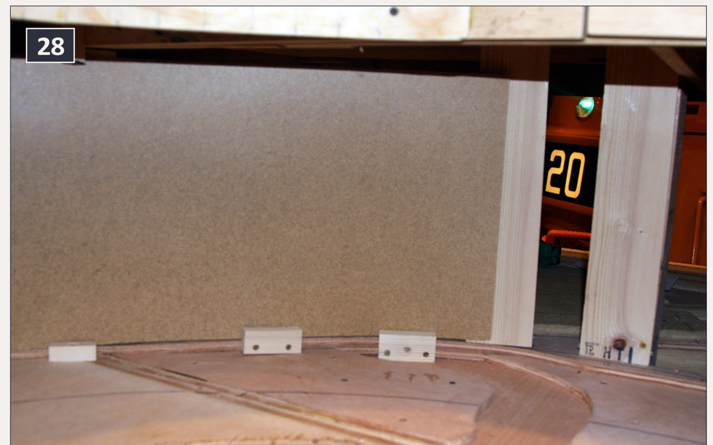
28: Backdrop supports at bottom and behind joint.
