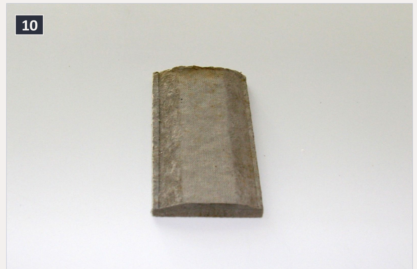
10: Celotex roadbed cross section.
