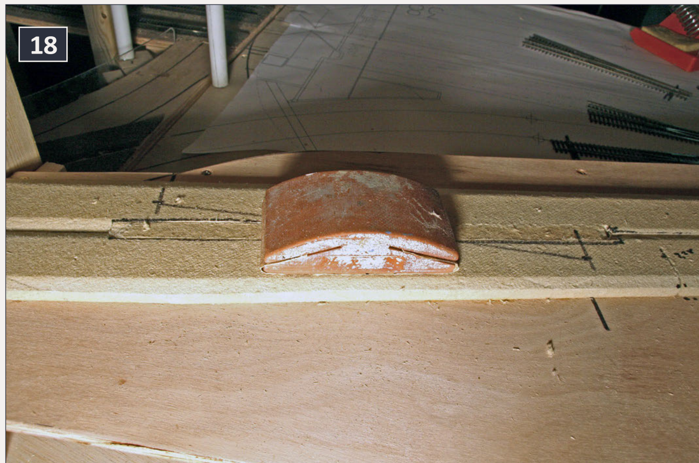
18: Sand the roadbed top smooth.
