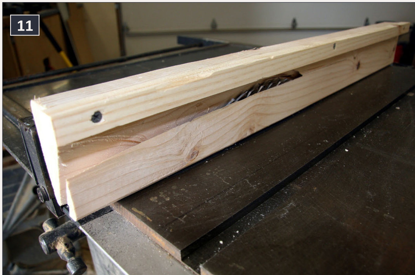
11: Jig for cutting roadbed.
